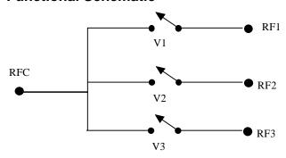
External blocking capacitors are required on all RF ports for positive control voltages. 100 pF recommended.
