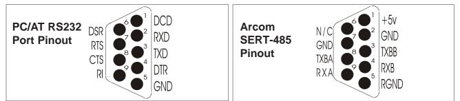
Cable connectors A and B can be of either pinout depending on links LK1-18. Cable connectors C and D are always RS232 pinout.
