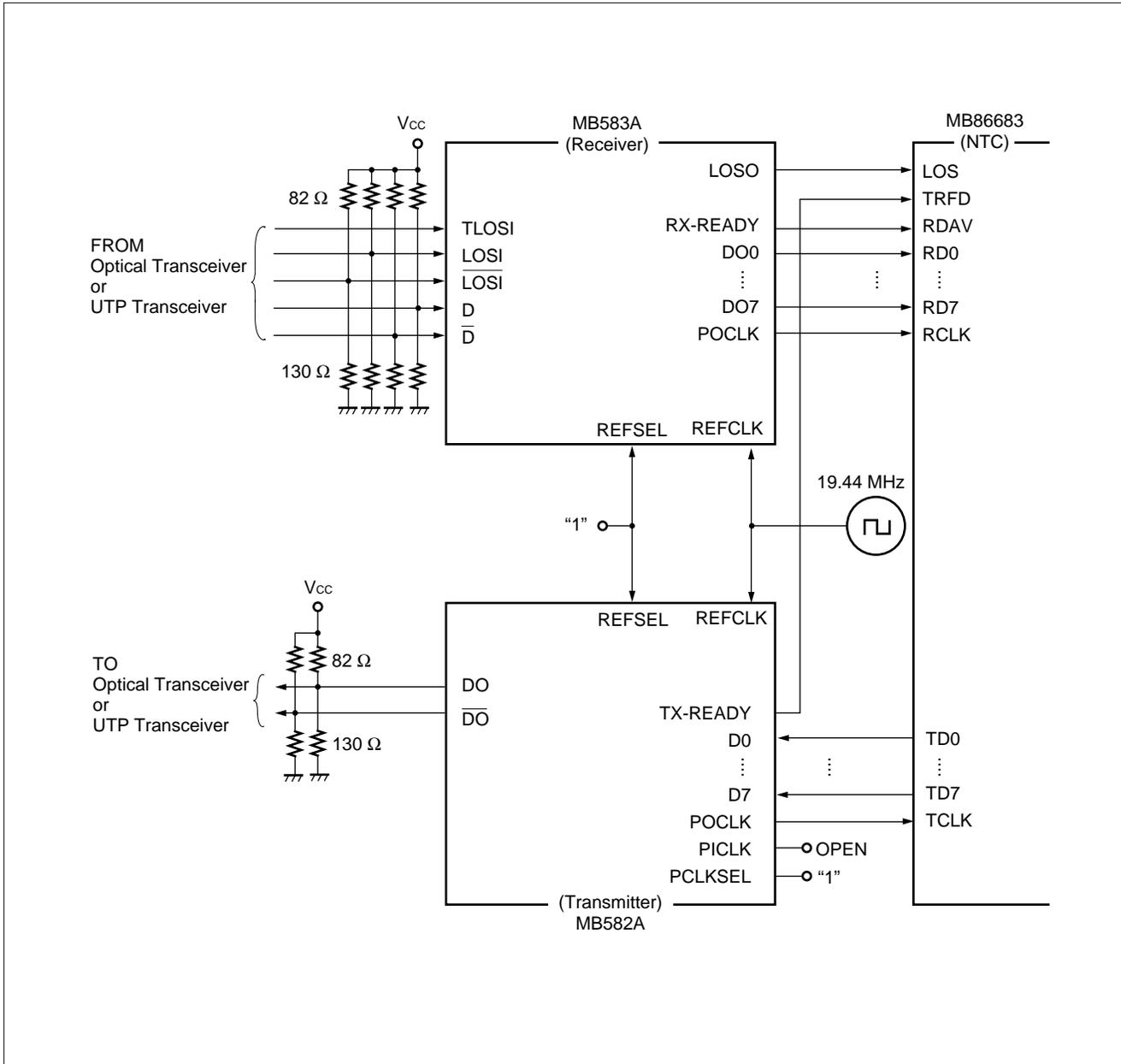
(2) When the MB582A uses PICKL = 19.44 MHz (without REFCLK) and the MB583A uses REFCLK = 19.44 MHz
