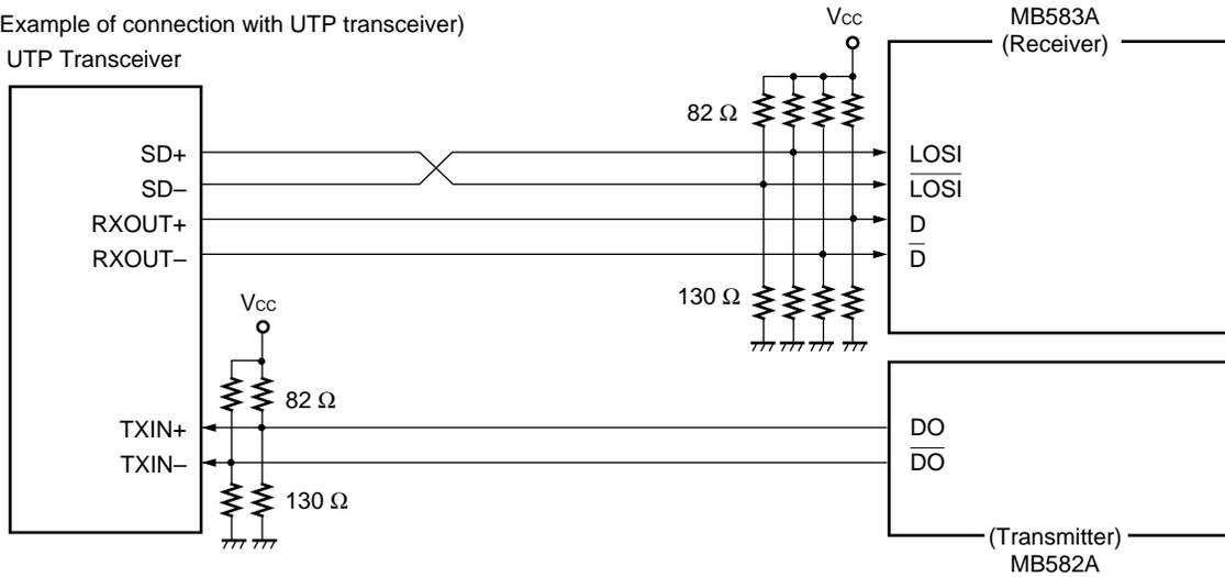
(Example of connection for a single input from optical transceiver to MB583A)
