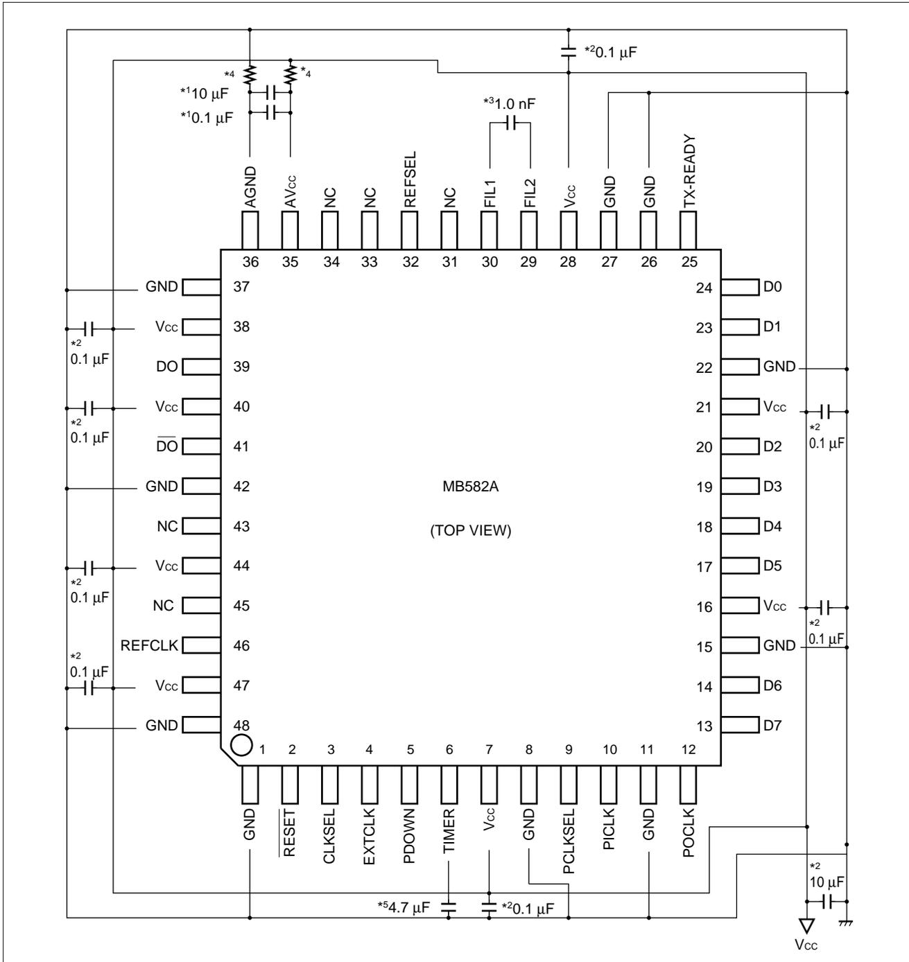
\*1: Bypass capacitor for power supply, connected between analog GND and analog V<sub>cc</sub>.
