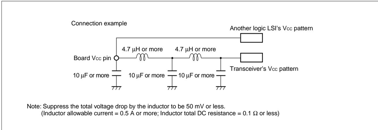
1-2. To prevent spike noise from another LSIs, add sufficient capacitance also to another LSIs (for example, 10  $\mu\text{F}$  for each of the LSIs).
