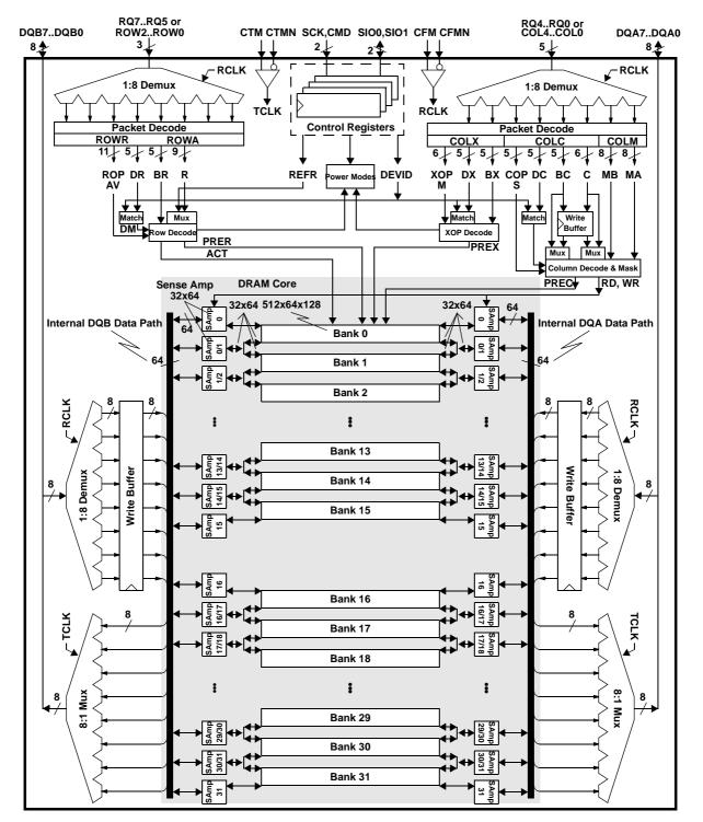
Figure 2: 128Mbit(256Kx16x32s) RDRAM Device Block Diagram
