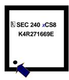
For consumer package, pin #1(ROW 1, COL A) is located at the A1 position on the top side and the A1 position is marked by the marker " $\bullet$  ".
