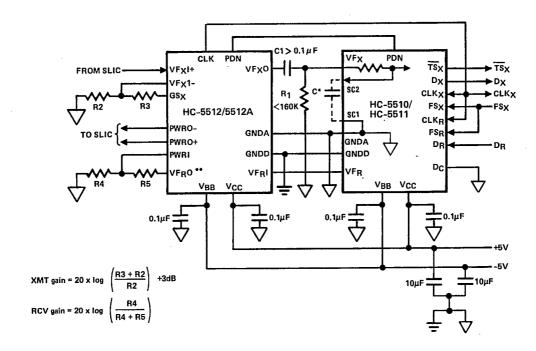
The power supply decoupling capacitors should be  $0.1\mu F$ . In order to take advantage of the excellent noise performance of the HC-5510/HC5511/HC-5512, care must be taken in board layout to prevent coupling of digital noise into the sensitive analog lines. The above application is configured for a fixed time slot mode of operation.
