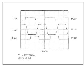
Figure 10. Loopback Test Result at 235kbps
