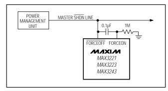
Figure 4. AutoShutdown with Initial Turn-On to Wake Up a Mouse or Another System
