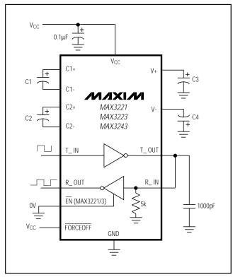
Figure 8. Loopback Test Circuit
