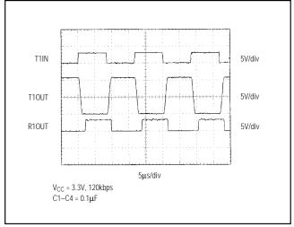
Figure 9. Loopback Test Result at 120kbps
