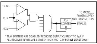
Figure 3a. MAX32\_ \_ Entering 1µA Supply Mode via AutoShutdown
