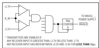
Figure 3b. MAX32\_ with Transmitters Enabled Using AutoShutdown
