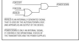
Figure 3c. AutoShutdown Logic
