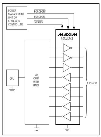
Figure 1. Interface Under Control of PMU
