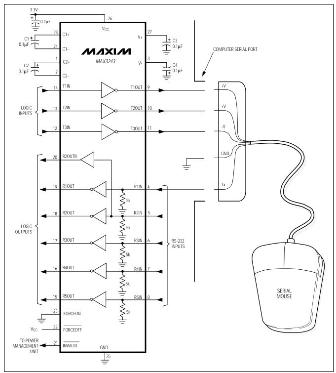
Figure 7b. Mouse Driver Test Circuit
