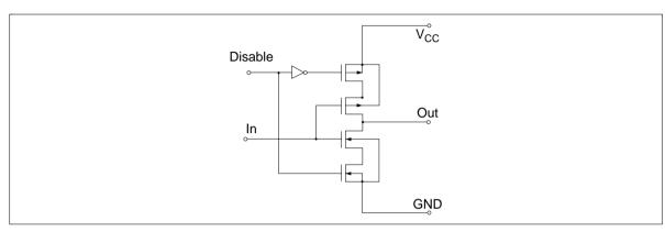
Figure 5 3-state Output Circuit
