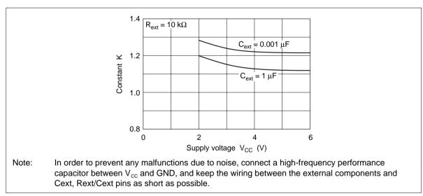
Figure 22 Constant K vs Supply Voltage
