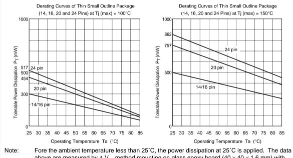
above are measured by  $\Delta$  V\_{\_{BE}} method mounting on glass epoxy board (40  $\times$  40  $\times$  1.6 mm) with 10% of wiring density. In the actual application, using conditions, ambient temperature and forced air-cooling conditions should be sufficiently examined.
