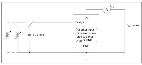
Figure 5 Latch-Up Immunity Test Circuit
