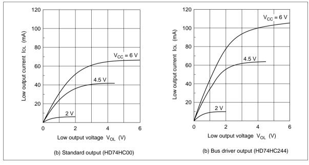
Figure 7 Output Current vs Voltage (Low Level)
