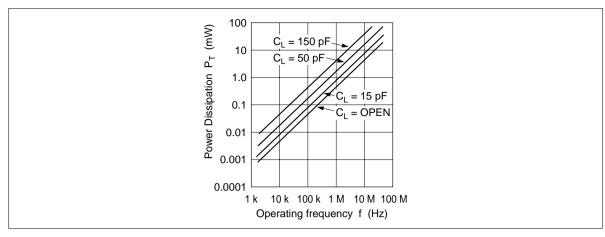
Figure 8 Power Dissipation VS. Operating Frequency
