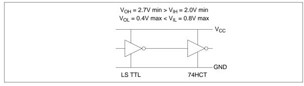
Figure 24 Interfacing LS-TTL to 74HCT
