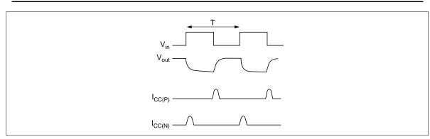
Figure 7 Operating Voltage and current of inverter circuit
