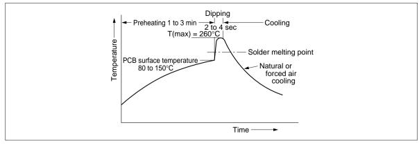
Figure 28 Temperature Profile of Dip Soldering
