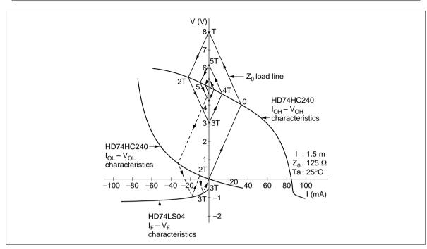
Figure 17 Bergeron Diagram Analysis of the Transmission Model
