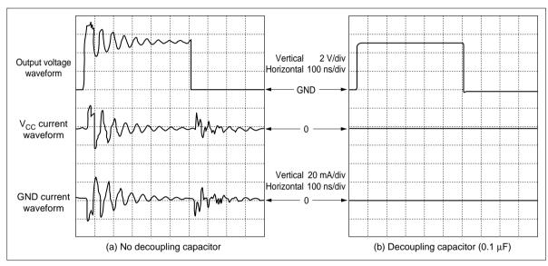
Figure 15 HD74HC00 Spike Current Waveform
