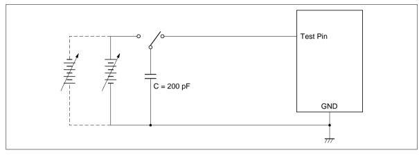
Figure 2 ESD Immunity Test Circuit
