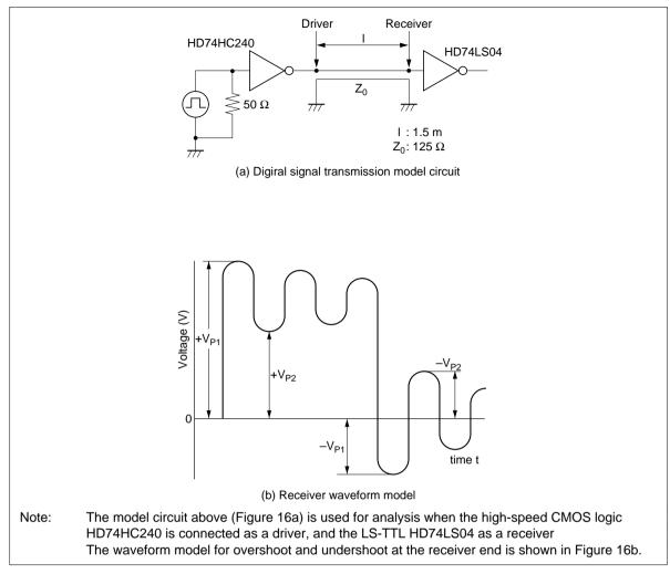
Figure 16 Digital Signal Transmission
