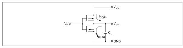
Figure 6 Inveter circuit
