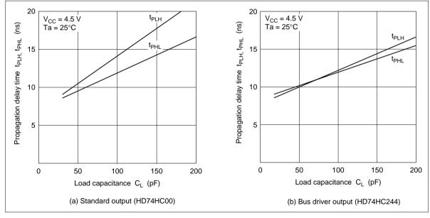
Figure 11 Propagation Delay Time vs Load Capacitance
