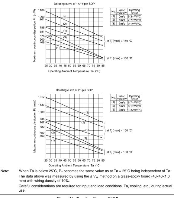
Figure 30 Derating Curves of SOP
