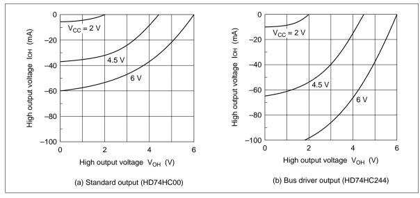
Figure 8 Output Current vs Voltage (High Level)
