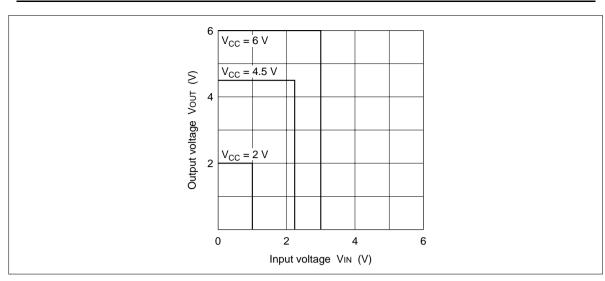
Figure 6 Output Voltage vs Input Voltage
