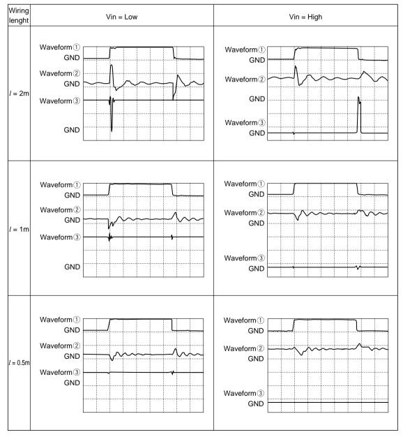
Figure 20 Crosstalk Noise Waveform (Driver: HD74HC240)
