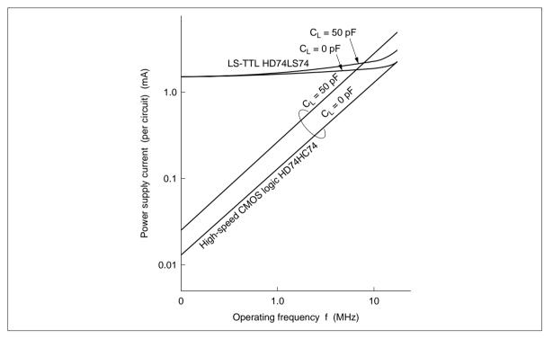
Figure 13 Operating Frequency vs Power Supply Current
