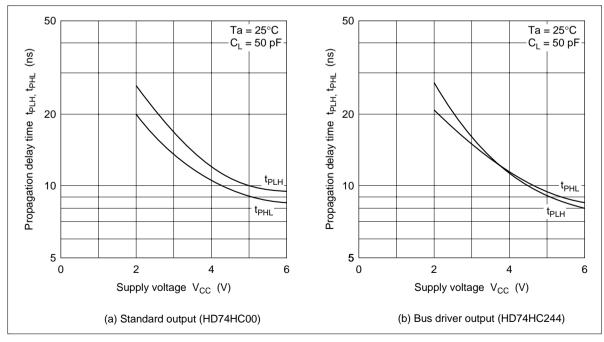
Figure 9 Propagation Delay Time vs Supply Voltage
