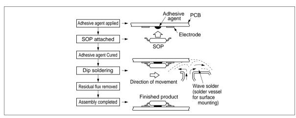
Figure 27 Process Flow for Dip Soldering SOP
