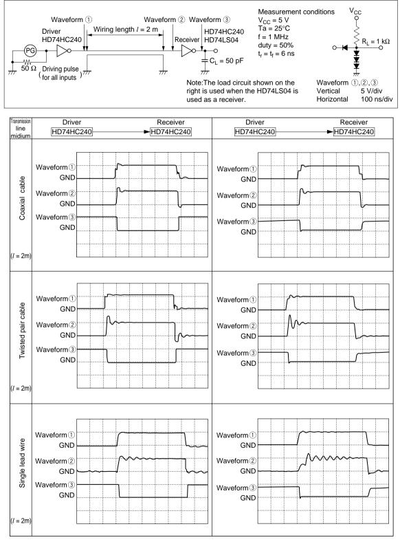
Figure 19 Reflection Ringing Waveforms (Driver: HD74HC240)
