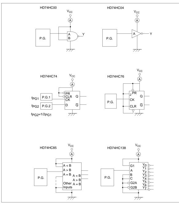
Figure 14 Measurement Circuits for Dynamic Power Supply Current
