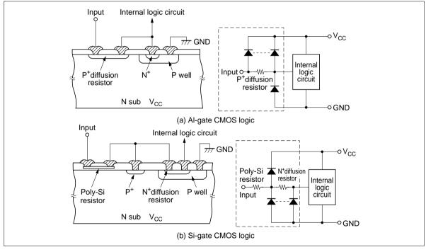
Figure 1 Input Protection Deevice and Equivalent Circuit
