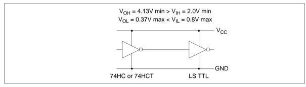
Figure 23 Interfacing HS-CMOS to LS-TTL
