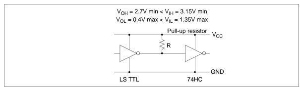
Figure 25 Interfacing LS-TTL to 74HC
