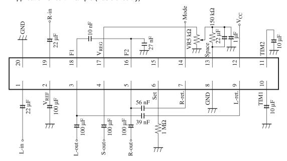
Note) When switching noise occurs at mode switching, insert a capacitor between pin 14 and GND.
