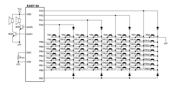
Note: In Easy 64 mode, only falling edge trigger can be used in input state
