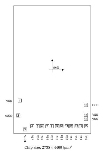
$\ast$  The IC substrate should be connected to VSS in the PCB layout artwork.
