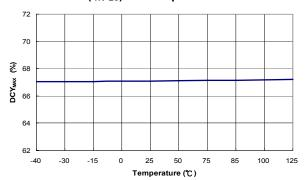
Figure 13. Maximum Duty Cycle (DCY<sub>MAX</sub>) vs. Temperature
