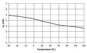
Figure 10. Supply Current Drawn from HV Pin (I<sub>HV</sub>) vs. Temperature
