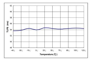
Figure 15. Delay Time of FB Pin Open-Loop Protection (t<sub>D-OLP</sub>) vs. Temperature
