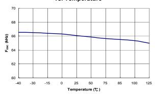
Figure 12. Frequency in Normal Mode (fosc) vs. Temperature
