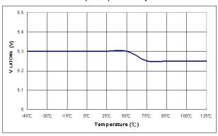
Figure 17. Latch-Off Threshold Voltage (V<sub>LATCHth</sub>) vs. Temperature
