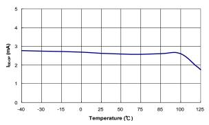
Figure 7. Operation Supply Current (I<sub>DD-OP</sub>) vs. Temperature
