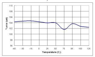
Figure 16. Output Current from LATCH Pin (I<sub>LATCH</sub>) vs. Temperature
