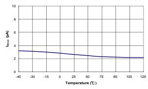
Figure 11. HV Pin Leakage Current After Startup (I<sub>HV-LC</sub>) vs. Temperature
