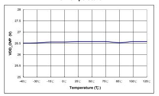
Figure 18.  $V_{DD}$  Over-Voltage Protection ( $V_{DD\text{-}OVP}$ ) vs. Temperature
