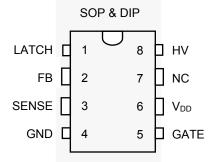
Figure 2. Pin Configuration (Top View)
