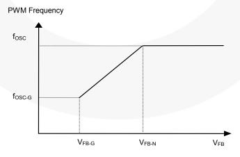
Figure 5. V<sub>FB</sub> vs. PWM Frequency
