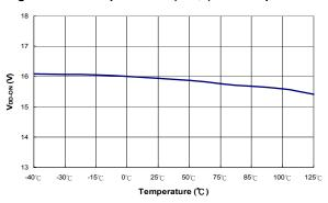
Figure 8. Start Threshold Voltage ( $V_{DD\text{-}ON}$ ) vs. Temperature
