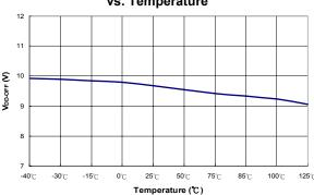
Figure 9. Minimum Operating Voltage ( $V_{DD\text{-}OFF}$ ) vs. Temperature
