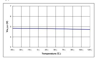
Figure 14. FB Open-Loop Trigger Level (V<sub>FB-OLP</sub>) vs. Temperature
