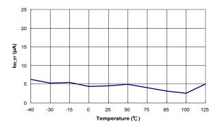
Figure 6. Startup Current (IDD-ST) vs. Temperature
