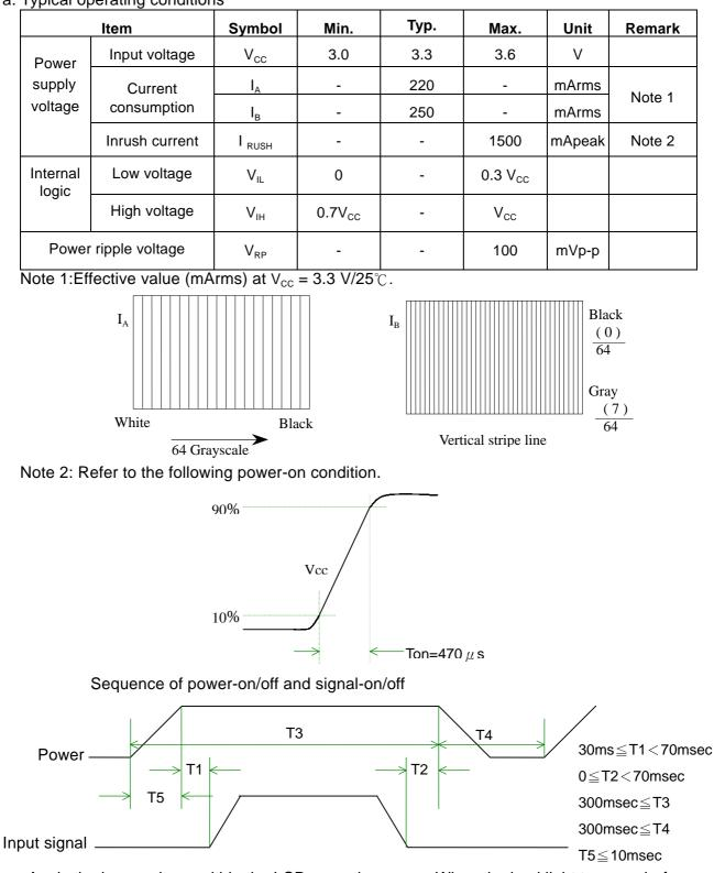
Apply the lamp voltage within the LCD operating range. When the backlight turns on before the LCD operation or the LCD turns off before the backlight turns off, the display may momentarily become abnormal.
