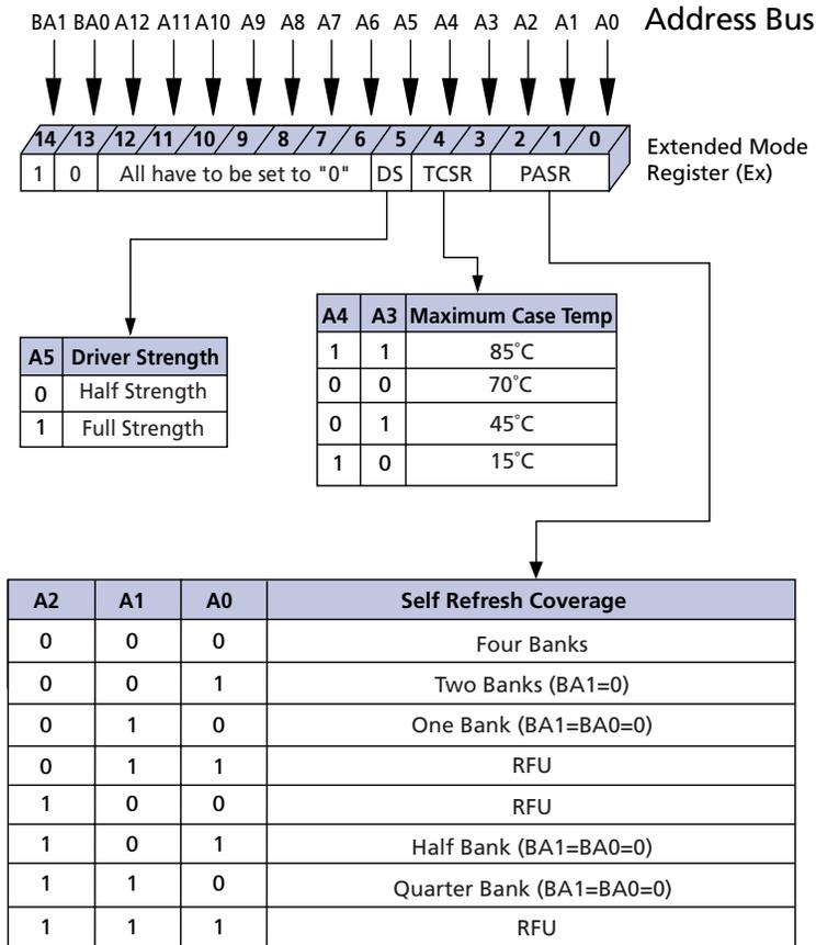
**NOTE:** 1. E14 and E13 (BA1 and BA0) must be "1, 0" to select the Extended Mode Register (vs. the base Mode Register).
