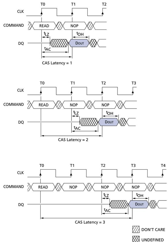
This is shown in Figure 7 for CAS latencies of two and three; data element  $n + 3$  is either the last of a burst of four or the last desired of a longer burst. The 256Mb SDRAM uses a pipelined architecture and therefore does not require the  $2n$  rule associated with a prefetch
