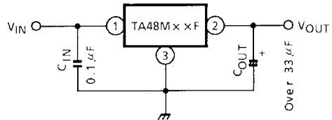
Connect the input terminal and GND, and the output terminal and GND, by capacitor respectively.
