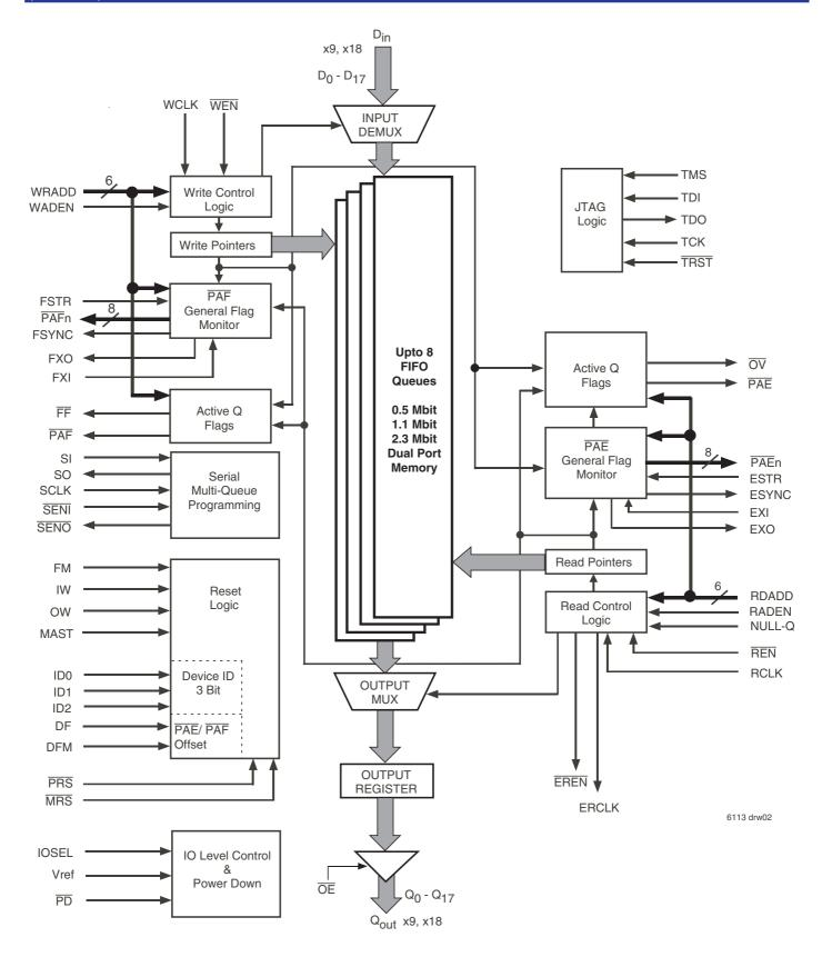
Figure 1. Multi-Queue Flow-Control Device Block Diagram
