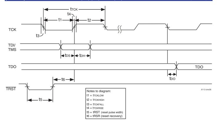
Figure 32. Standard JTAG Timing
