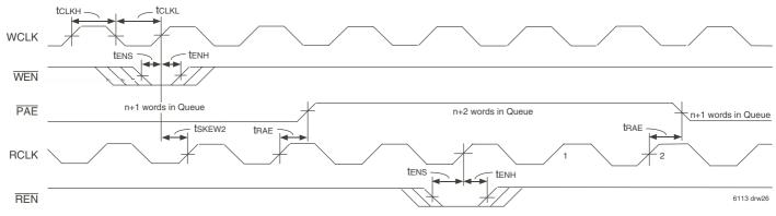
1. The waveform here shows the PAE flag operation when no queue switches are occurring and a queue selected on both the write and read ports is being written to then read from at the almost empty boundary.
