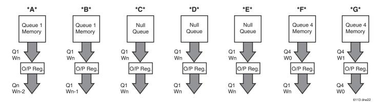
Figure 18. Null Queue Flow Diagram
