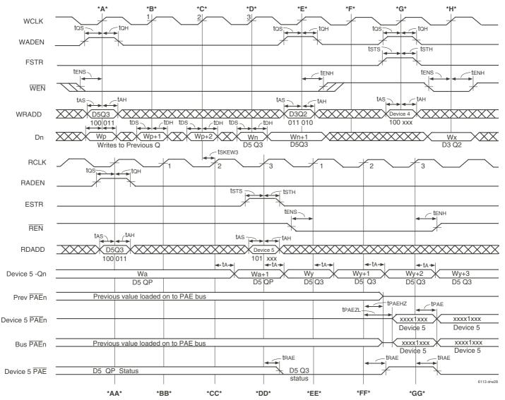
\*A\* Q3 of Device 5 is selected for write operations.
