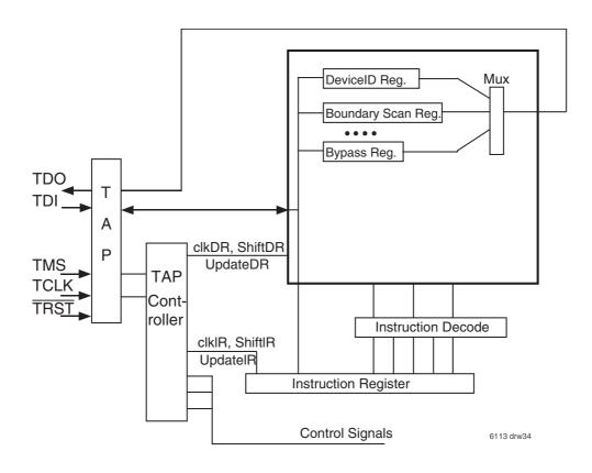
Figure 30. Boundary Scan Architecture
