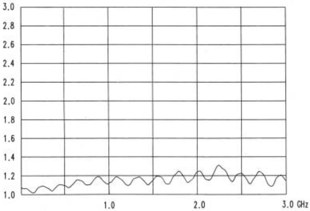
Typical data using fully assembled and connected GT16-1P-HU and the GT5-1S-HU.
