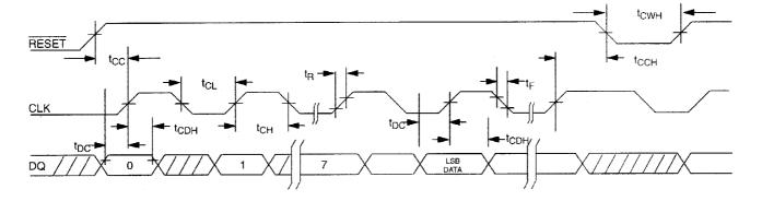
NOTE:  $t_{CL}$ ,  $t_{CH}$ ,  $t_R$ , and  $t_F$  apply to both read and write data transfer.
