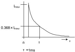
1pulse/3s (7000 cycle) I<sub>FRM</sub> = 150 A (C<sub>M</sub> = 500μF)
