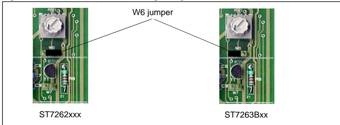
If you are using the analog trimmer, select the installed ST7 device using jumper W6 as shown in [Figure 2](#). This ties the analog trimmer to the PA0 I/O port of the ST7262xxx devices and to the PB0 port of the ST7263Bxx devices. Any other analog input pin on the microcontroller can be used by removing the W6 jumper and wiring the center pin of W6 to the analog input.
