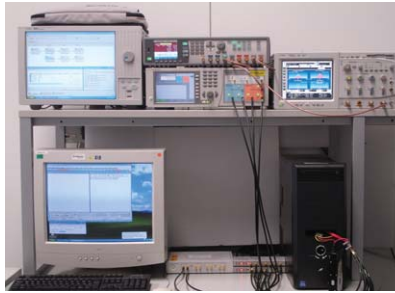
Figure 7. Automated SATA test station – user-friendly, full automation is achieved by supporting the Agilent N4915A-005 SATA switch
