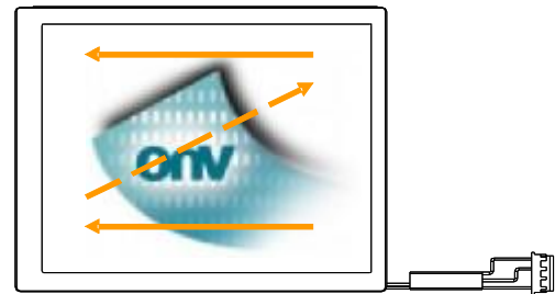
Fig. 2 Reverse scan (Pin4, DPS = High)
