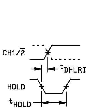
FIGURE 5. Channel selection timing.
