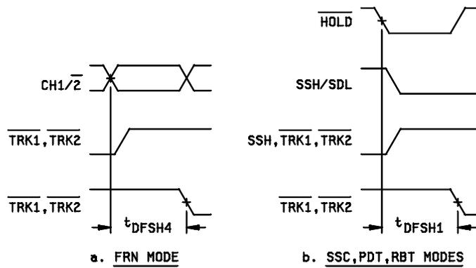
FIGURE 4. Control output timing.
