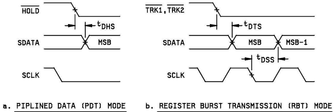
FIGURE 8. Data transmission timing.
