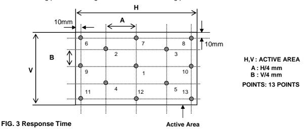
The response time is defined as the following figure and shall be measured by switching the input signal for "black" and "white".
