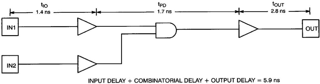
**Sequential Delay Example** (Load = 30 pF, K=1, Fanout=1)
