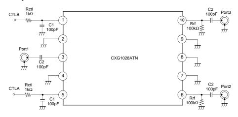
When using the CXG1028ATN, the following external components should be used:
