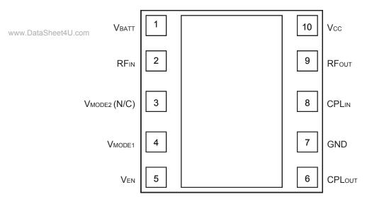
Figure 2: Pinout (X-ray Top View)
