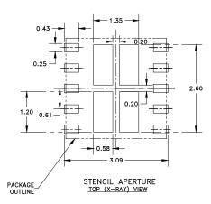
Figure 6: Recommended PCB Layout Information
