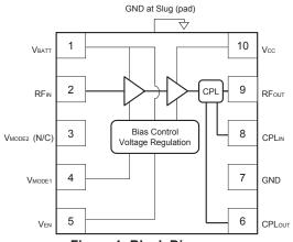
Figure 1: Block Diagram
