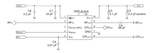
Figure 3: Application Circuit Schematic
