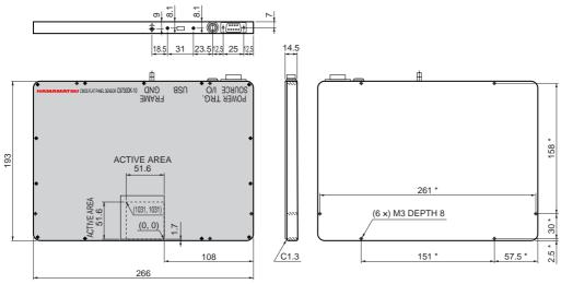
Top cover material including window is carbon fiber (1.0 mm thickness). Weight: 1.3 kg
