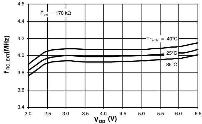
**Figure 71.** System Clock versus  $V_{DD}$
