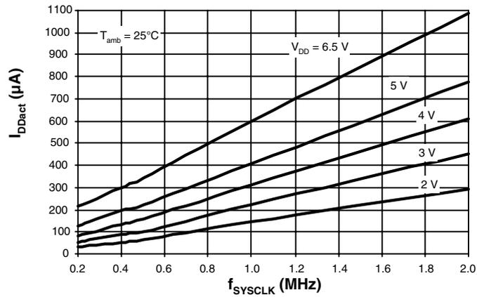
**Figure 64. Power-down Supply Current versus Frequency**
