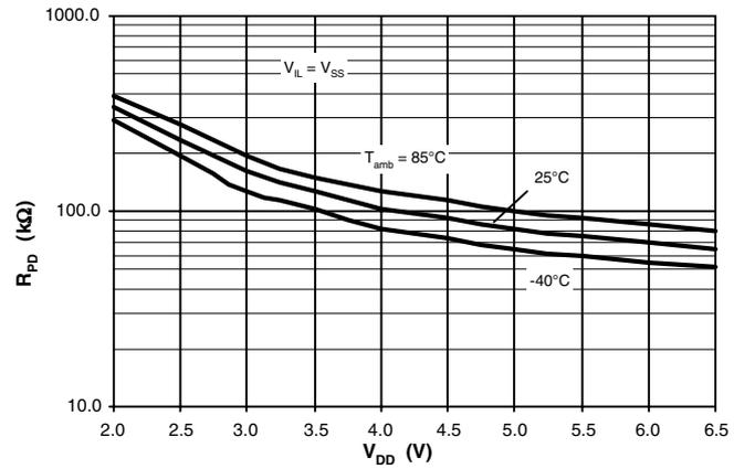
Figure 79. Strong Pull-down Resistor versus  $V_{DD}$
