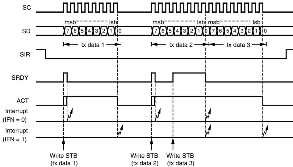
**Figure 46.** Example of 8-bit Synchronous Receive Operation
