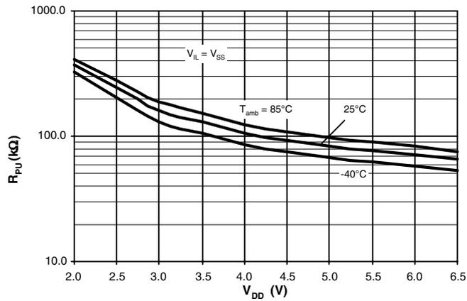
**Figure 76.** Strong Pull-up Resistor versus  $V_{DD}$
