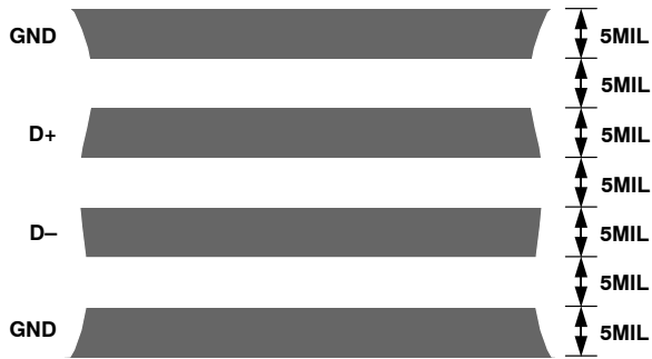
Figure 23. Typical Arrangement of Signal Tracks
