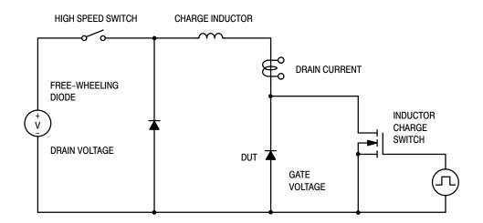
Figure 10. Simplified UIS Test Circuit
