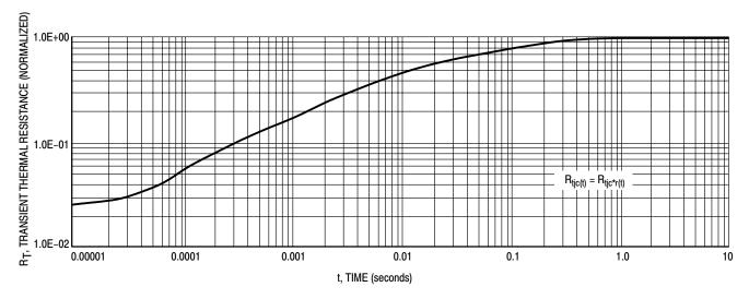
Figure 9. Typical Thermal Response
