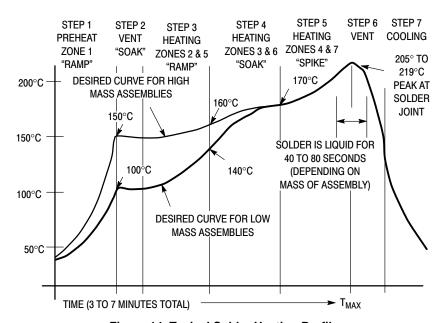
Figure 14. Typical Solder Heating Profile
