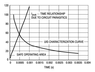
Figure 13. DUT Peak Reverse and Circuit Parasitic Inductance Current versus Time
