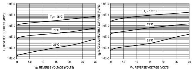
**Figure 3. Typical Reverse Current**
