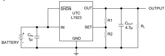
Figure 2. Adjustable Output Using External Feedback Resistors
