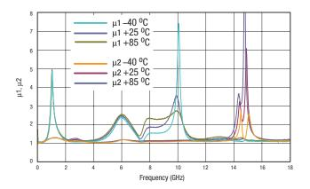
Figure 10. Stability vs Frequency Over Temperature ( $P_{IN} = -20 \text{ dBm}$ )
