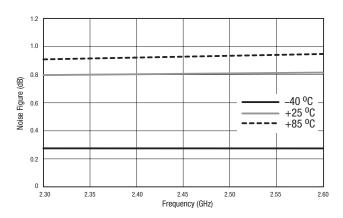
Figure 7. Noise Figure vs Frequency Over Temperature
