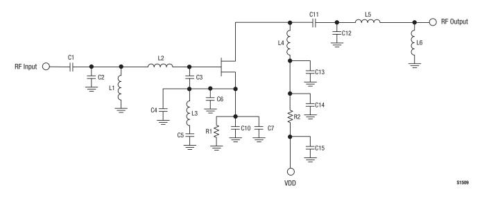
Figure 12. SKY65053-377LF Evaluation Board Schematic
