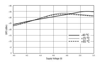
Figure 8. OIP3 vs Supply Voltage (f = 2.4 GHz, Tone Spacing = 10 MHz, Pout = +5 dBm/Tone)
