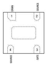
Figure 2. SKY65053-377LF Pinout – 4-Pin QFN (Top View)
