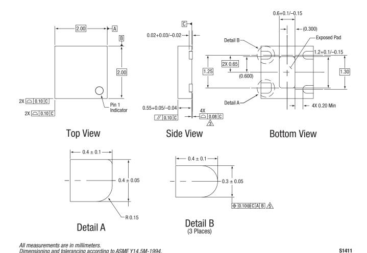
Figure 15. SKY65053-377LF 4-Pin QFN Package Dimensions
