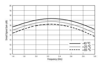
Figure 3. Small Signal Gain vs Frequency Over Temperature (PIN = -20 dBm)
