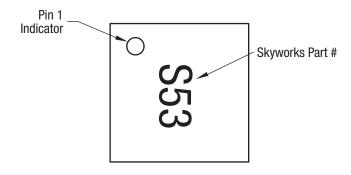
Figure 14. Typical Case Markings (Top View)
