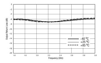
Figure 6. Output Return Loss vs Frequency Over Temperature (PiN = -20 dBm)
