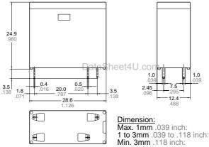
**Tolerance** ±0.1 ±.004 ±0.2 ±.008 ±0.3 ±.012 PC board pattern (Bottom view) **4-1.3 dia** .071 dia 20.0 3.5 .138DataShe
