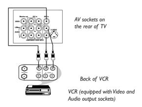
You can view the playback of VCR tapes (Video Disc players, camcorders, etc.) by using the AUDIO and VIDEO INPUT sockets on the rear of the TV.
