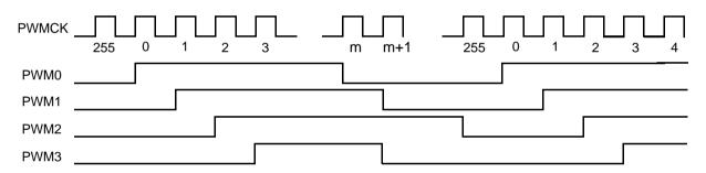
FIGURE 9. 5 Channel PWM Output Rising Edges Are Separated by One PWMCK
