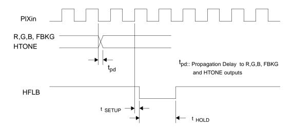
FIGURE 12. Output and HFLB Timing to Pixel Clock
