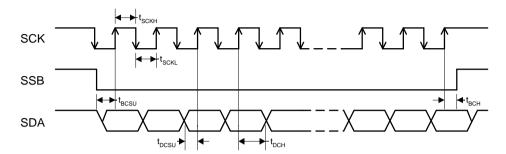
FIGURE 10. Data interface timing(SPI)
