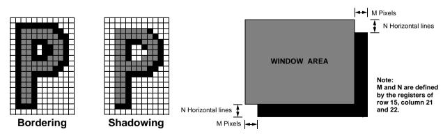
FIGURE 8. Character Bordering and Shadowing and Shadowing on Window
