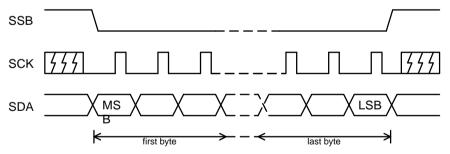
FIGURE 1. Data Transmission Protocol (SPI)
