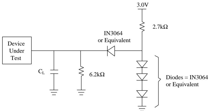
**Note :**  $C_L = 100pF$  including jig capacitance
