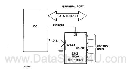
Most of the control lines resulting from the decoding of F < 0-3 > are used to control the flow of the data to and from the Peripheral Port Data lines. These data lines are used when an IOC executes certain programmed I/O instructions or when it performs Data Channel Breaks. The following sections explain how the Peripheral Port reacts during the execution of these instructions and commands.
