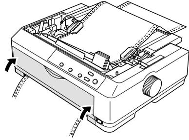
If you have the LQ-2090, remove the sub cover from the front cover before replacing the front cover. Be sure to reattach the sub cover when you want to print from a different paper source.
