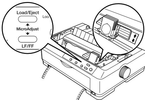
5. Press the Pause button to exit Micro Adjust mode.
