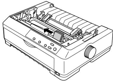
4. Remove the new ribbon cartridge from the package. The black plastic ribbon guide is held in place on top of the cartridge with a small tab. To release it, hold the sides of the ribbon guide and gently disconnect it. (Do not remove the ribbon guide from the ribbon, however.)
