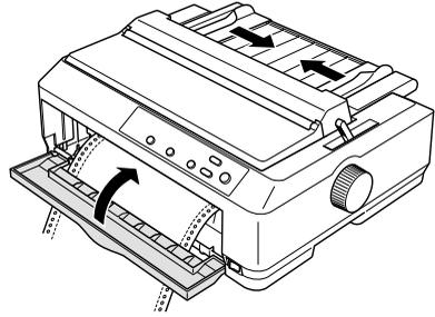
12. Turn on the printer. When the printer receives data, it automatically loads the paper and starts printing.
