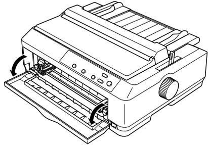
2. If you have the LQ-2090, remove the sub cover from the front cover. (If it is difficult to remove, you can temporarily remove the front cover and then separate the sub cover from it.)
