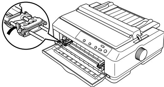
5. Slide the left sprocket approximately 0.5 inch (12 mm) from the far left position and pull the blue lever forward to lock it in place. Then slide the right sprocket to match the width of your paper, but do not lock it.
