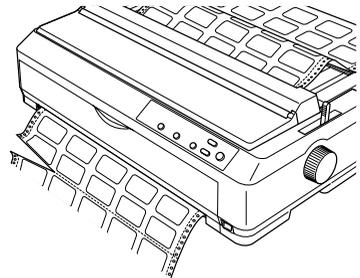
2. Hold down the LF/FF button to eject the remaining labels from the printer.
