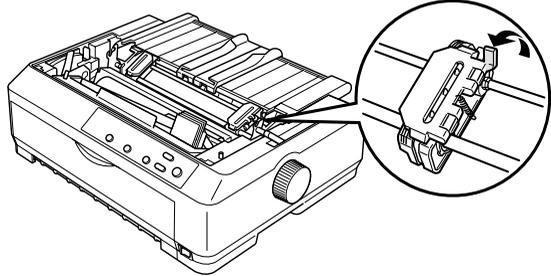
4. Slide the left sprocket approximately 0.5 inch (12 mm) from the far left position and push the lever back to lock it in place.
