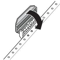
8. Slide the right sprocket to remove any slack in the paper, then lock it in place.
