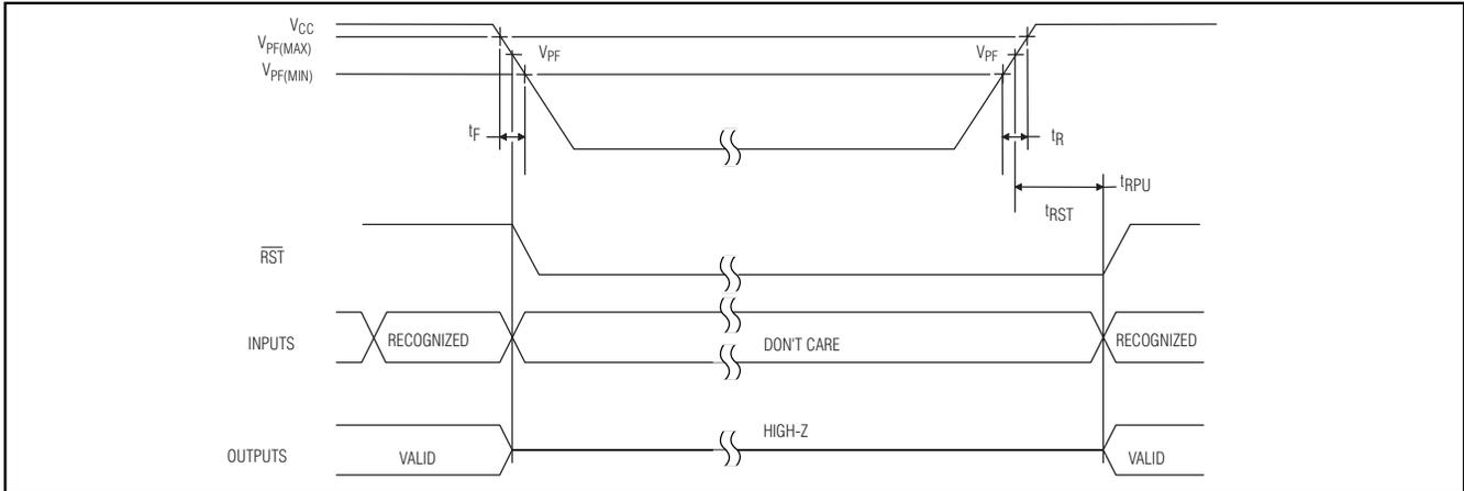
Figure 2. Power-Up/Power-Down Timing
