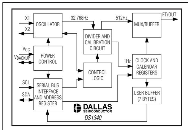
Figure 5. Functional Diagram
