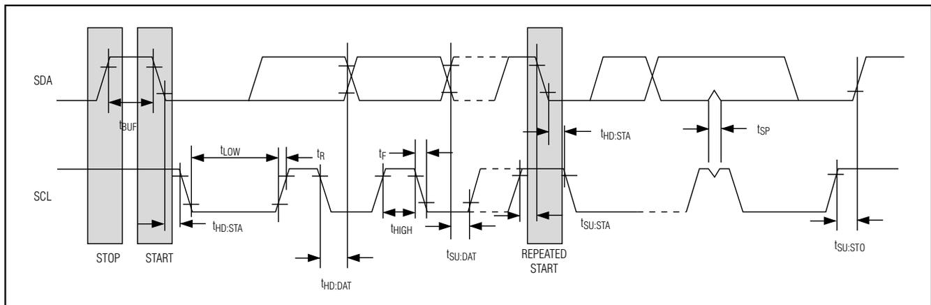
Figure 1. Data Transfer on 2-Wire Serial Bus
