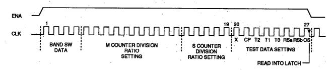
(2) Test mode bit set up
