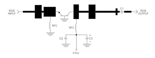
T = 20 MIL TFE, Er = 2.55 C1,C2 = 62pF CHIP ATC "A" C3 = 10MFD @ 35V RFC = 4 turns 22 wire 1/16" I.D.
