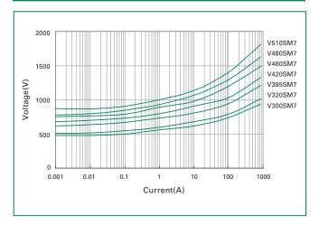
NOTE: If pulse ratings are exceeded, a shift of  $V_{N(DC)}$  (at specified current) of more than  $\pm 10\%$  could result. This type of shift, which normally results in a decrease of  $V_{N(DC)}$ , may result in the device not meeting the original published specifications, but it does not prevent the device from continuing to function, and to provide ample protection.
