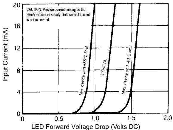
Figure 6. Input Characteristics
