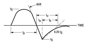
Figure 14. Diode Reverse Recovery Waveform
