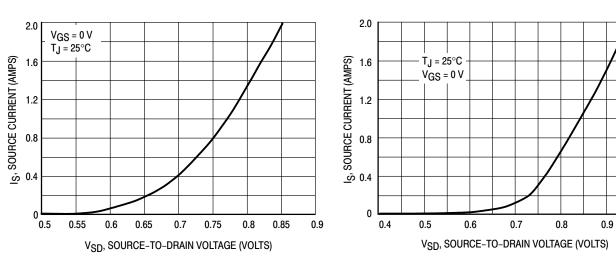
Figure 10. Diode Forward Voltage versus Current
