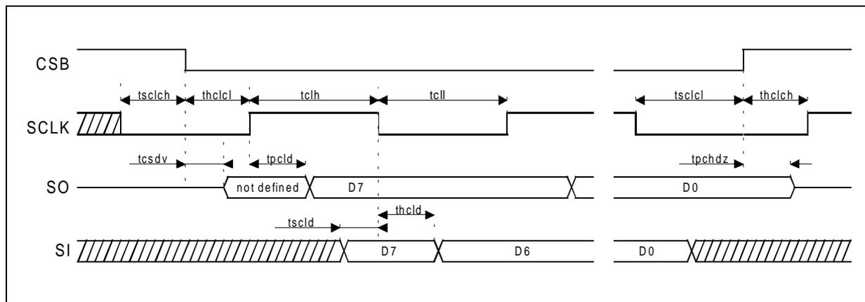
The SPI register data are transferred to the output latch at rising CSB edge. The digital filter between CSB and the output latch ensures that the data are transferred only after 8 SCLK cycles or multiple of 8 SCLK cycles since the last CSB falling edge. The CSB changes only at low SCLK.
