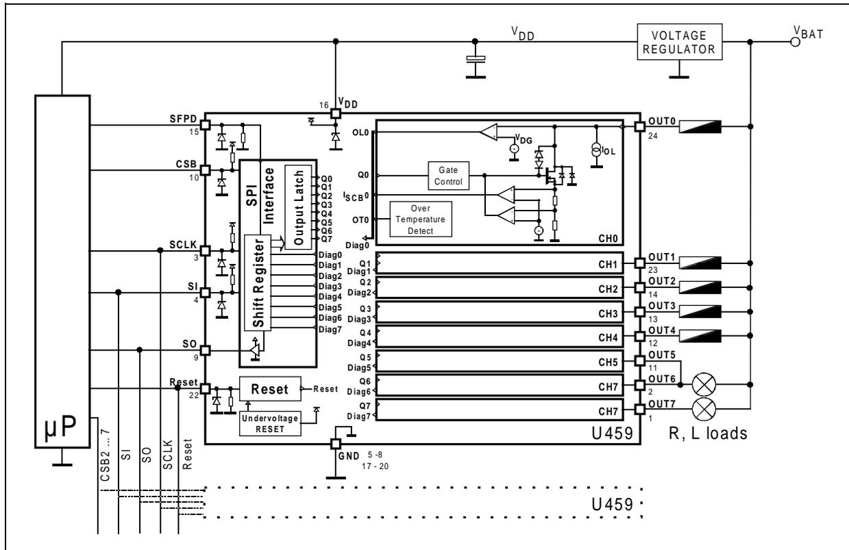
For higher current driving capability more outputs of the same kind can be paralleled. In this case the maximum flyback energy should not exceed the limit value for single output.
