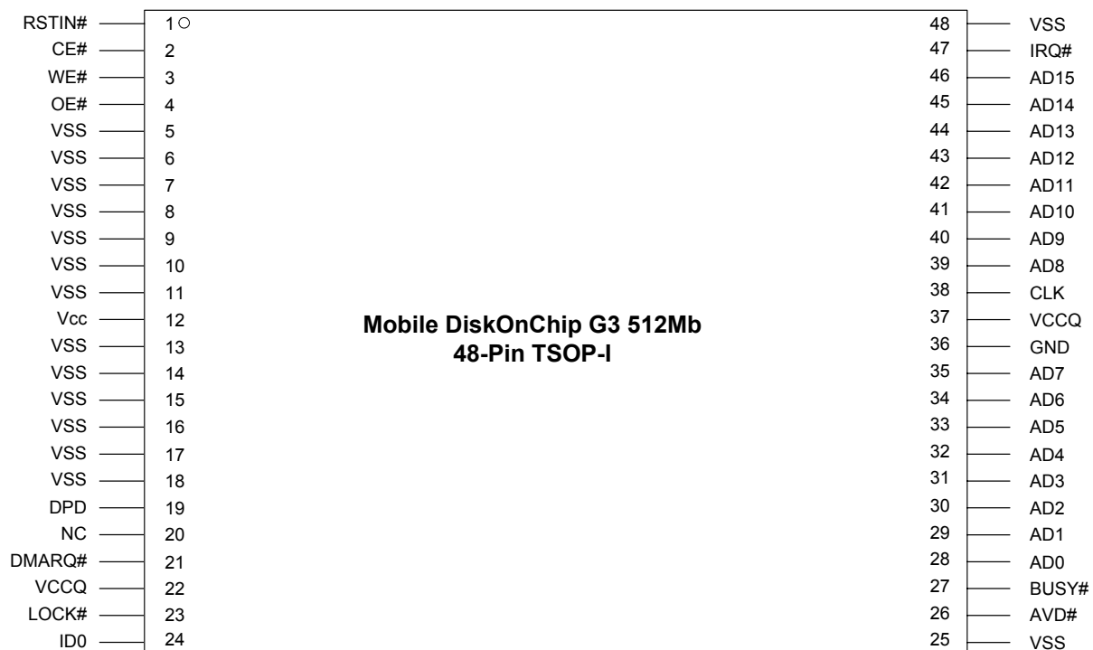
Figure 6: Pinout for Multiplexed Interface (Mobile DiskOnChip 512Mb TSOP-I Package)
