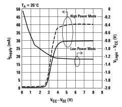
Figure 5. Typical Supply Current &  $V_{Logic}\mbox{ vs.}$  Supply Voltage.
