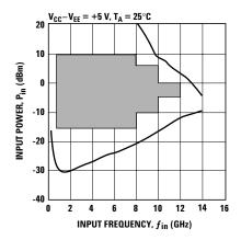
Figure 4. Typical Input Sensitivity Window.
