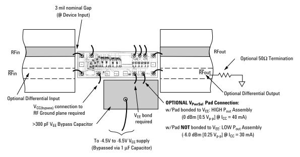
Figure 3. Assembly Diagrams.
