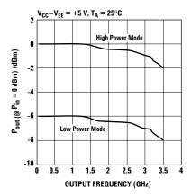
Figure 7. Typical Output Power vs. Output Frequency,  $f_{\rm out}$  (GHz).
