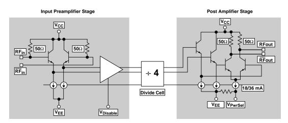
Figure 1. HMMC-3024 Simplified Schematic.
