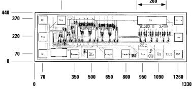
Figure 2. Pad Locations and Chip Dimensions.
