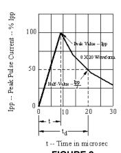
FIGURE 2 Pulse Wave Form
