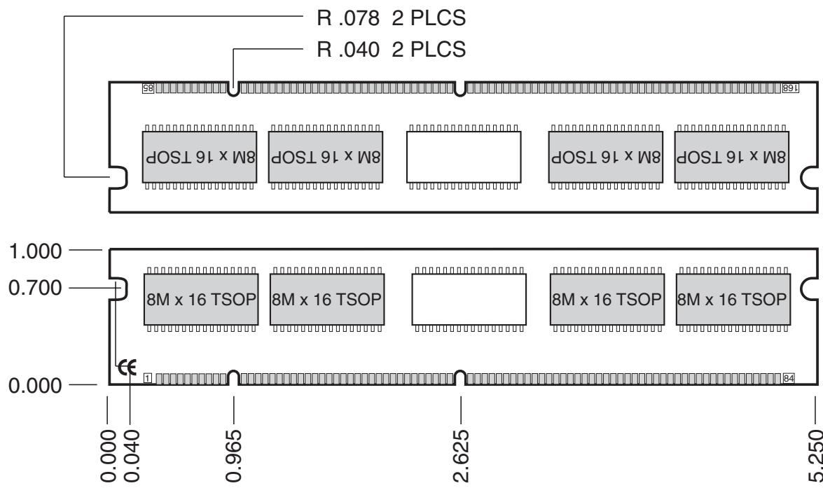
Figure 1: KVR100X64C2L/128 168-Pin SDRAM Module
