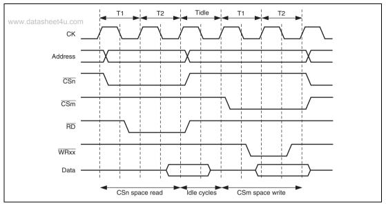
Figure 9.7 Example of Idle Cycle Insertion
