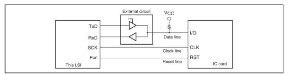
Figure 13.21 Example of Pin Connections for Smart Card Interface
