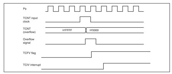
Figure 11.66 TCIV Interrupt Setting Timing
