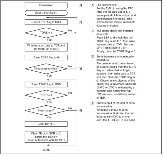
Figure 13.11 Sample Multiprocessor Serial Transmission Flowchart
