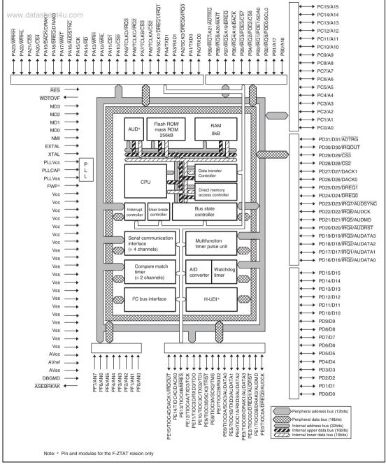
Figure 1.2 Block Diagram of SH7145
