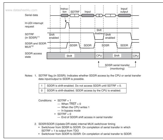
Figure 22.2 Data Input/Output Timing Chart (1)
