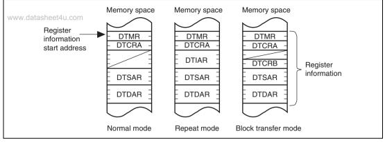
Figure 8.3 DTC Register Information Allocation in Memory Space
