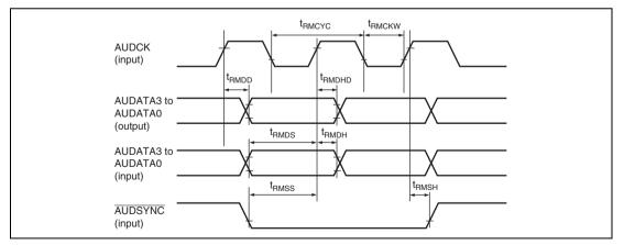
Figure 26.29 RAM Monitor Timing
