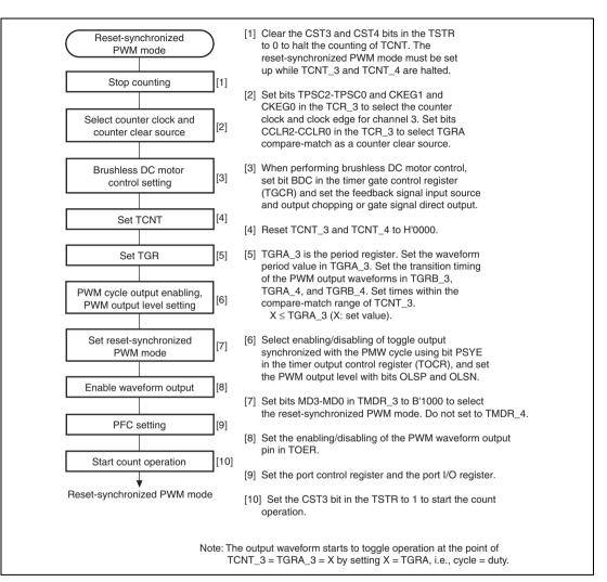
Figure 11.30 Procedure for Selecting Reset-Synchronized PWM Mode
