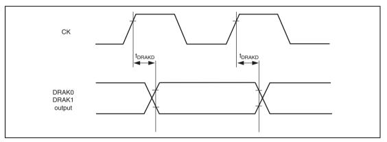
Figure 26.14 DRAK Output Delay Time
