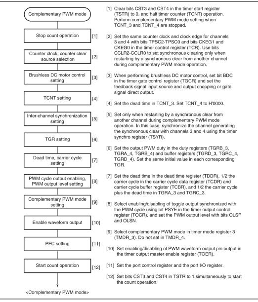
Figure 11.33 Example of Complementary PWM Mode Setting Procedure
