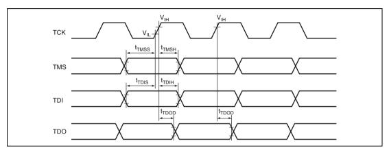
Figure 26.26 H-UDI Input/Output Timing
