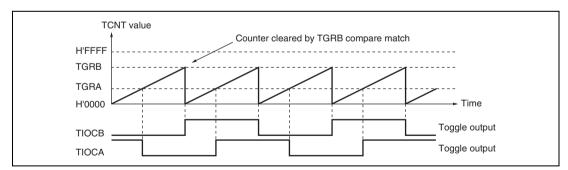
Figure 11.8 Example of Toggle Output Operation
