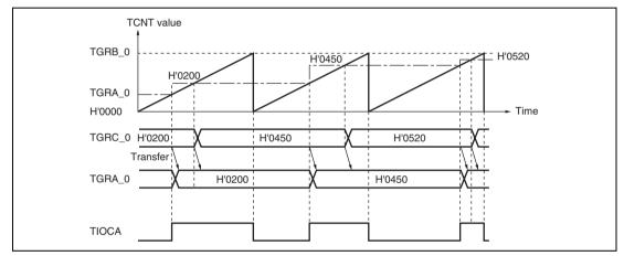
Figure 11.16 Example of Buffer Operation (1)
