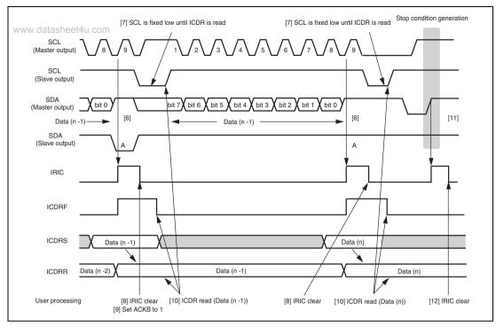
Figure 14.19 An Example of the Timing of Operations in Slave Receive Mode 2 (MLS = 0, HNDS = 1)
