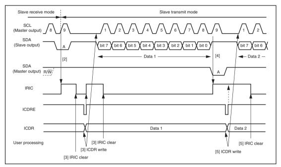
Figure 14.24 An Example of the Timing of Operations in Slave Transmit Mode (MLS = 0)
