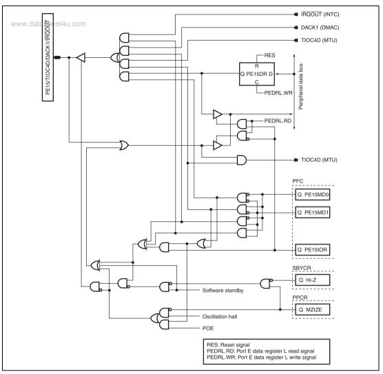
Figure D.42 PE15/TIOC4D/DACK1/IRQOUT
