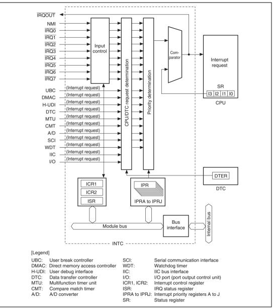
Figure 6.1 INTC Block Diagram
