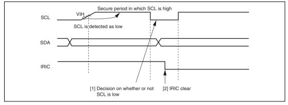
Figure 14.33 Timing for Clearing IRIC Flag When WAIT = 1
