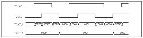
Figure 11.19 Example of Cascaded Operation
