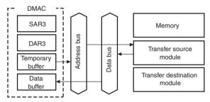
The value in the temporary buffer is taken as the address, and data is read from the transfer source module to the data buffer.
