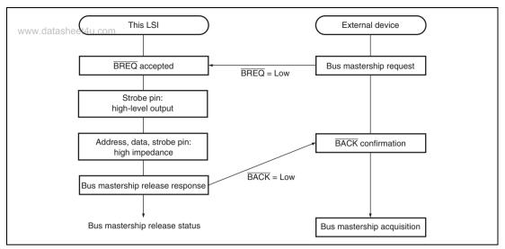
Figure 9.9 Bus Mastership Release Procedure
