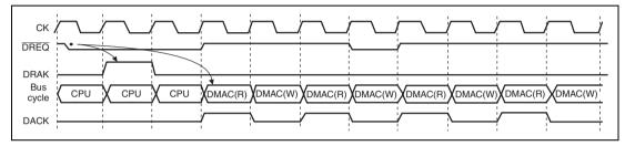
Figure 10.22 Burst Mode, Dual Address and Edge Detection
