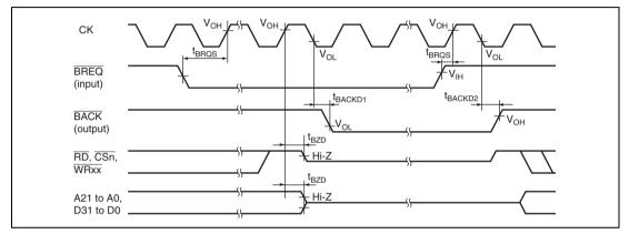
Figure 26.8 Bus Release Timing
