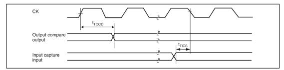
Figure 26.15 MTU Input/Output timing
