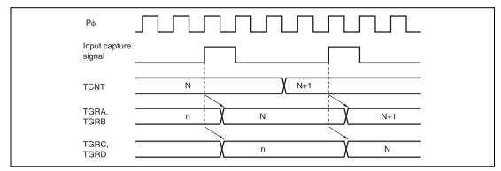
Figure 11.63 Buffer Operation Timing (Input Capture)
