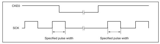
Figure 13.29 Timing for Fixing Clock Output Level
