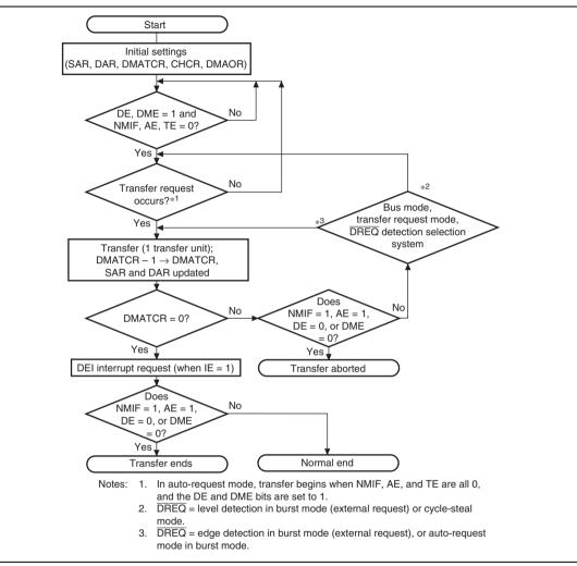
Figure 10.2 DMAC Transfer Flowchart
