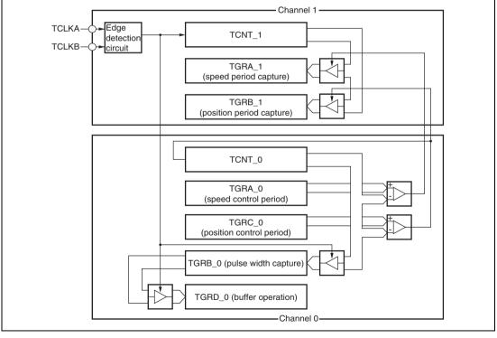
Figure 11.29Phase Counting Mode Application Example
