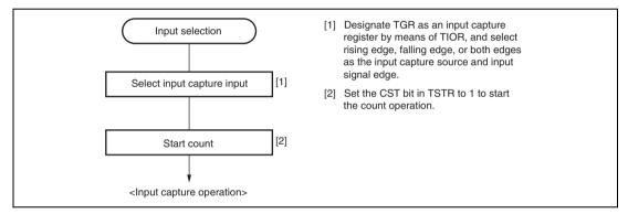
Figure 11.9 Example of Input Capture Operation Setting Procedure
