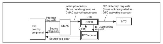
Figure 8.2 Activating Source Control Block Diagram
