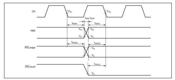
Figure 26.6 Interrupt Signal Input Timing
