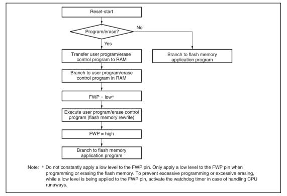
Figure 19.6 Programming/Erasing Flowchart Example in User Program Mode
