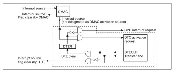
Figure 6.6 Interrupt Control Block Diagram
