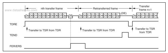
Figure 13.26 Retransfer Operation in SCI Transmit Mode
