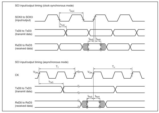
Figure 26.20 SCI Input/Output Timing
