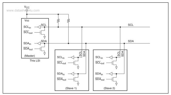
Figure 14.2 Example of the Connection of I<sup>2</sup>C Bus Interfaces (This LSI Is the Master Device)
