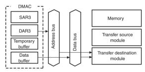
The DAR3 value is taken as the address, and the value in the data buffer is written to the transfer destination module.
