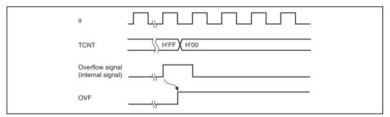
Figure 12.4 Timing of Setting OVF
