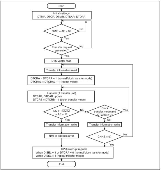
Figure 8.5 DTC Operation Flowchart
