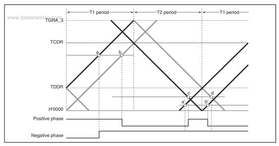
Figure 11.42 Example of Complementary PWM Mode Waveform Output (3)
