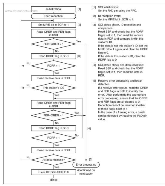
Figure 13.13 Sample Multiprocessor Serial Reception Flowchart (1)
