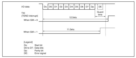
Figure 13.27 TEND Flag Generation Timing in Transmit Operation
