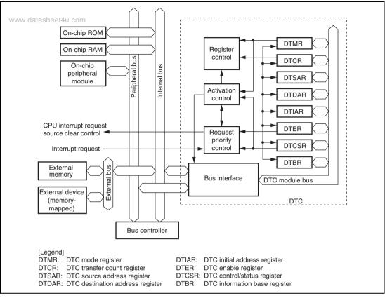
Figure 8.1 Block Diagram of DTC
