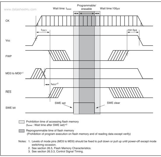
Figure 19.12 Power On/Off Timing (User Program Mode)
