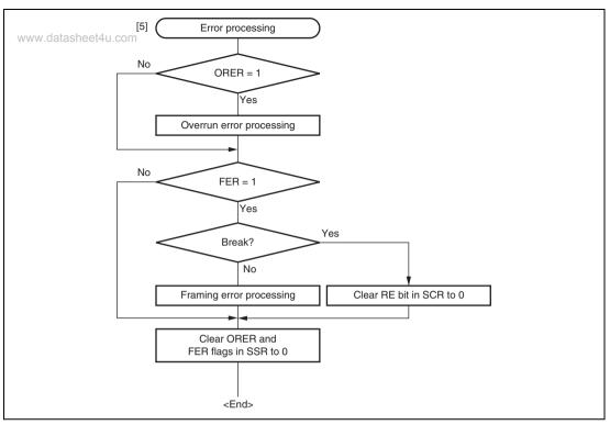
Figure 13.13 Sample Multiprocessor Serial Reception Flowchart (2)
