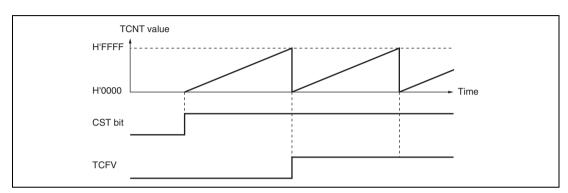
Figure 11.4 illustrates free-running counter operation.
