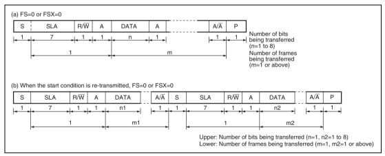
Figure 14.3 I<sup>2</sup>C Bus Data Format (I<sup>2</sup>C Bus Format)
