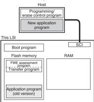
Flash memory initialization The programming/erase program in RAM is executed, and the flash memory is initialized (to H'FF). Erasing can be performed in block units, but not in byte units.  Programming/erase control program transfer When user program mode is entered, user software confirms this fact, executes transfer program in the flash memory, and transfers the programming/erase control program to RAM.
