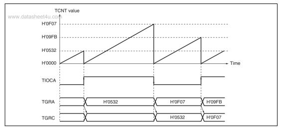
Figure 11.17 Example of Buffer Operation (2)
