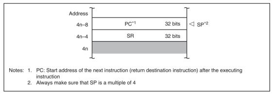
Figure 6.4 Stack after Interrupt Exception Processing
