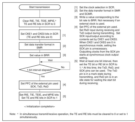
Figure 13.5 Sample SCI Initialization Flowchart
