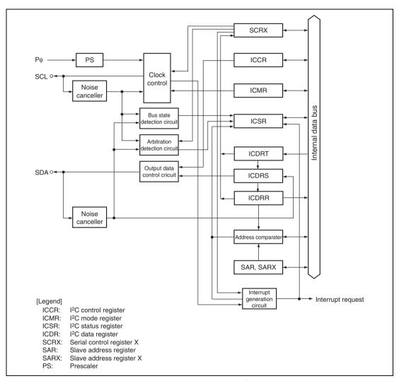
Figure 14.1 A Block Diagram of the I<sup>2</sup>C Bus Interface
