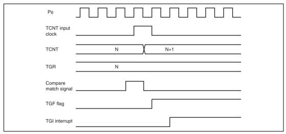
Figure 11.64 TGI Interrupt Timing (Compare Match)
