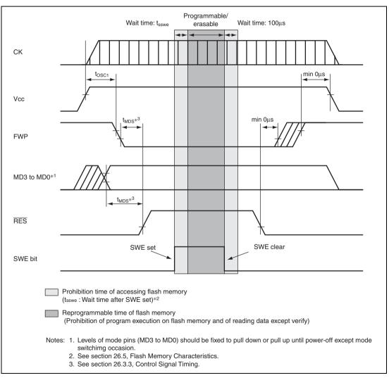
Figure 19.11 Power On/Off Timing (Boot Mode)
