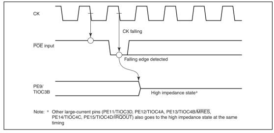
Figure 11.117 Falling Edge Detection Operation
