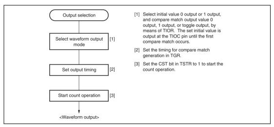
Figure 11.6 Example of Setting Procedure for Waveform Output by Compare Match
