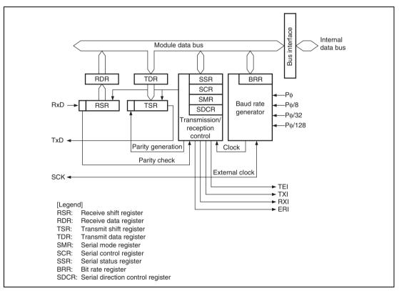
Figure 13.1 Block Diagram of SCI
