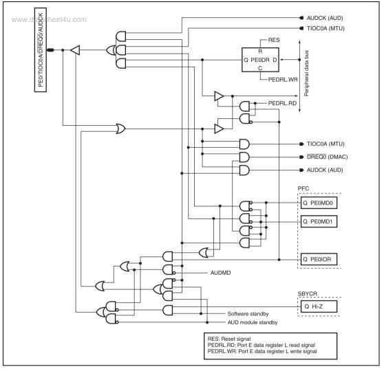
Figure D.46 PE0/TIOC0A/DREQ0/AUDCK
