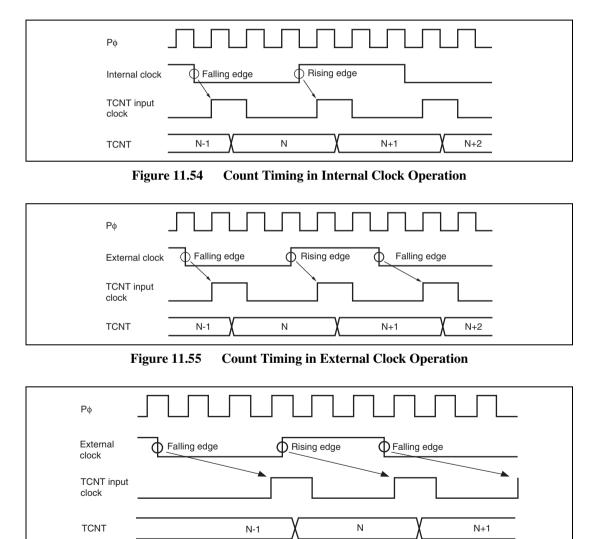
Figure 11.56 Count Timing in External Clock Operation (Phase Counting Mode)
