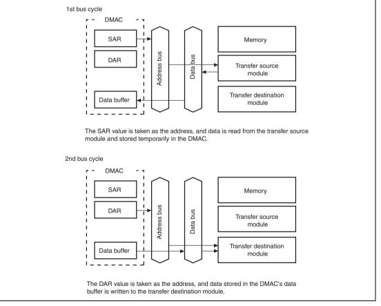
Figure 10.6 Direct Address Operation during Dual Address Mode
