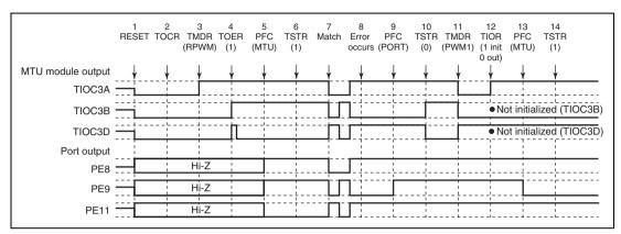
Figure 11.111 Error Occurrence in Reset-Synchronous PWM Mode, Recovery in PWM Mode 1
