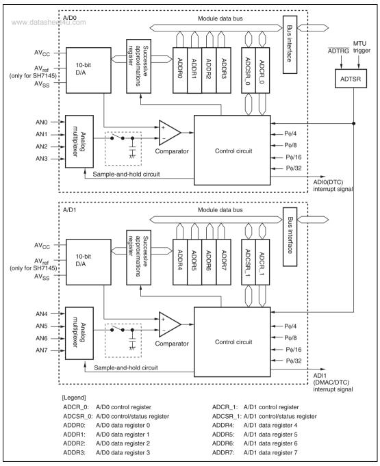
Figure 15.1 Block Diagram of A/D Converter
