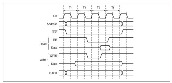
Figure 9.6 CS Assert Period Extension Function
