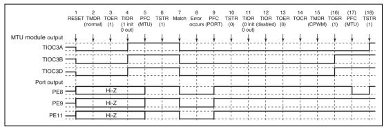
Figure 11.89 Error Occurrence in Normal Mode, Recovery in Complementary PWM Mode
