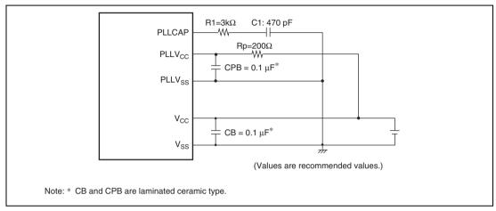
Figure 4.6 Recommended External Circuitry around PLL
