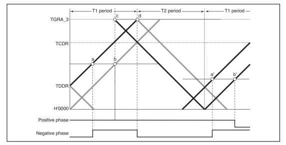
Figure 11.43 Example of Complementary PWM Mode 0% and 100% Waveform Output
