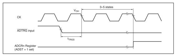
Figure 26.23 External Trigger Input Timing
