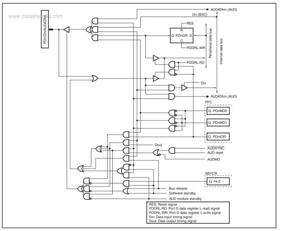
Figure D.24 PDn/Dn/AUDATAm
