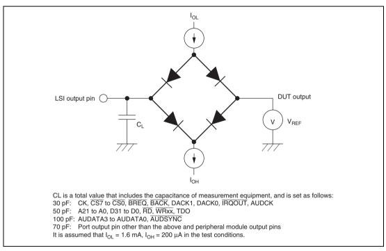
Figure 26.1 Output Load Circuit
