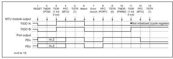
Figure 11.103 Error Occurrence in Phase Counting Mode, Recovery in PWM Mode 2
