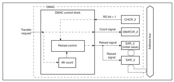
Figure 10.24 Source Address Reload Function
