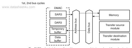
The SAR3 value is taken as the address, memory data is read, and the value is stored in the temporary buffer. Since the value read at this time is used as the address, it must be 32 bits. When external connection data bus is 16 bits, two bus cycles are required.
