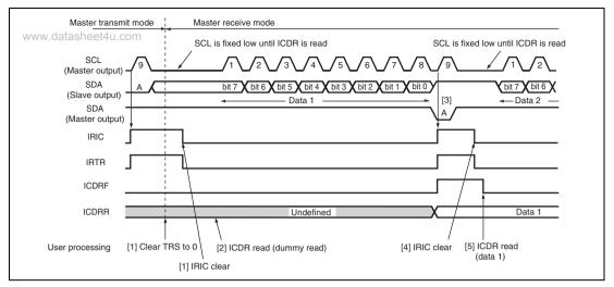
Figure 14.11 An Example of the Timing of Operations in Master Receive Mode (MLS = WAIT = 0, HNDS = 1)
