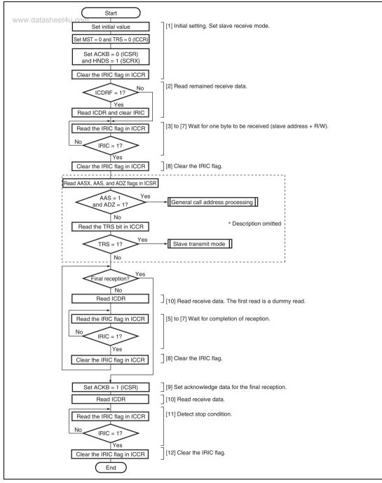
Figure 14.17 Example: Flowchart of Operations in the Slave Receive Mode (HNDS = 1)
