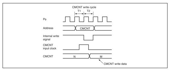
Figure 16.7 CMCNT Word Write and Increment Contention
