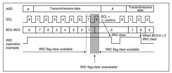
Figure 14.32 IRIC Flag Clear Timing on WAIT Operation
