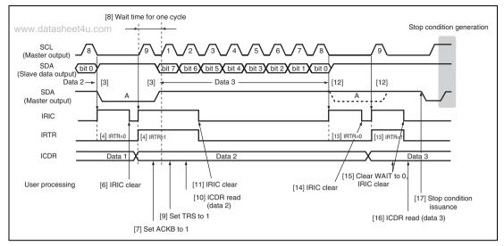
Figure 14.16 An Example of the Stop Condition Issuance Timing in Master Receive Mode (MLS = ACKB = 0, WAIT = 1)
