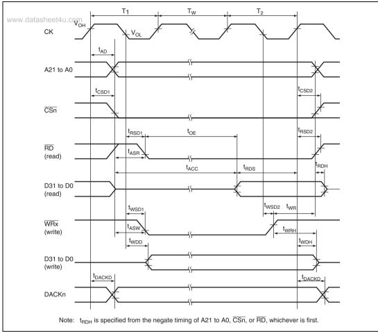
Figure 26.10 Basic Cycle (One Software Wait)
