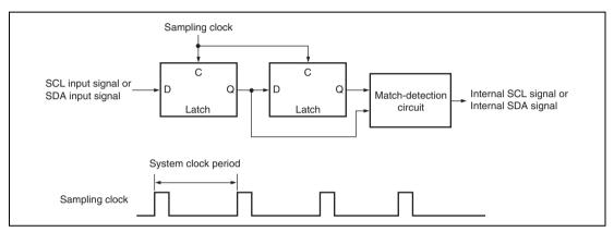
Figure 14.28 Block Diagram of the Noise Canceller
