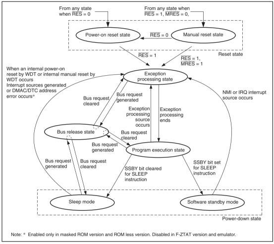
Figure 2.4 Transitions between Processing States
