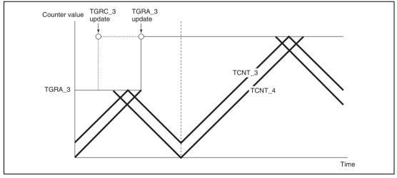
Figure 11.36 Example of PWM Cycle Updating
