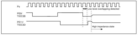
Figure 11.116Output-Level Detection Operation
