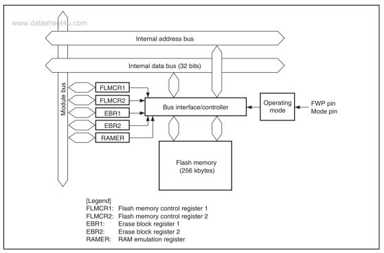
Figure 19.1 Block Diagram of Flash Memory
