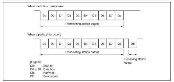
Figure 13.22 Normal Smart Card Interface Data Format
