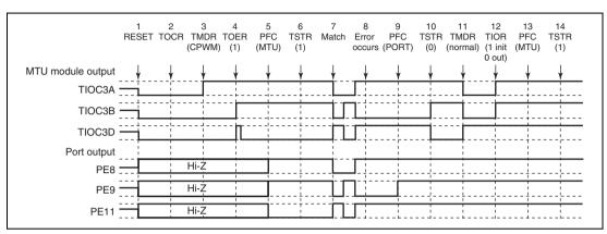
Figure 11.110 Error Occurrence in Reset-Synchronous PWM Mode, Recovery in Normal Mode
