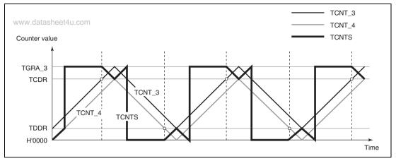
Figure 11.34 Complementary PWM Mode Counter Operation
