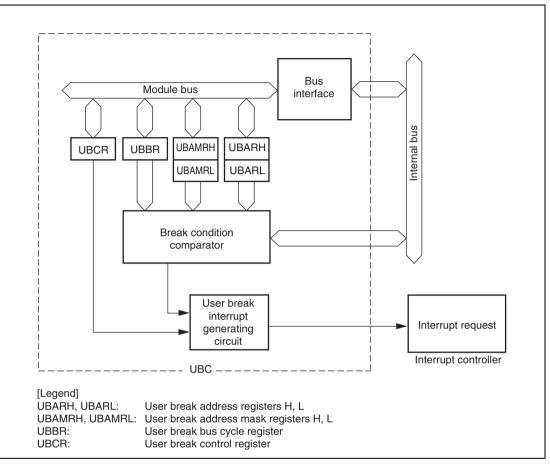
Figure 7.1 User Break Controller Block Diagram
