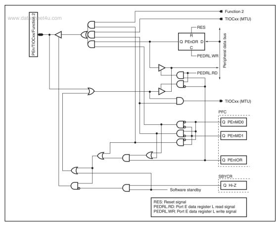
Figure D.35 PEn/TIOCxx/Function 2
