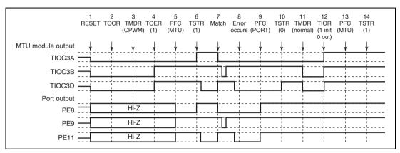
Figure 11.105 Error Occurrence in Complementary PWM Mode, Recovery in Normal Mode
