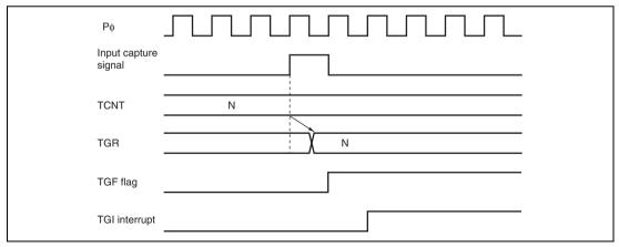
Figure 11.65 TGI Interrupt Timing (Input Capture)
