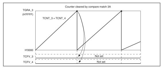
Figure 11.82 Reset Synchronous PWM Mode Overflow Flag
