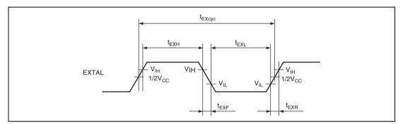
Figure 26.3 EXTAL Clock Input Timing
