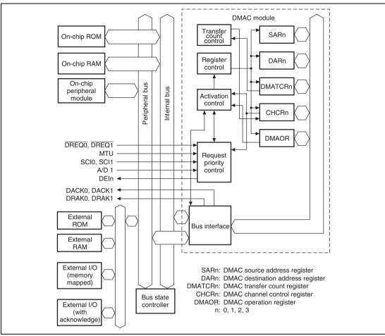
Figure 10.1 DMAC Block Diagram
