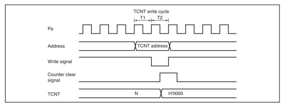
Figure 11.71 Contention between TCNT Write and Clear Operations
