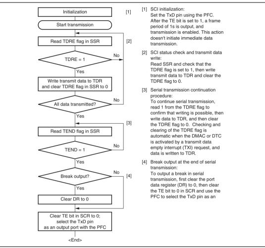
Figure 13.7 Sample Serial Transmission Flowchart
