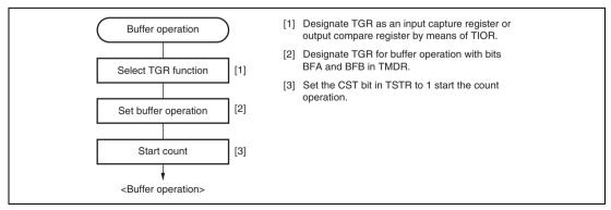
Figure 11.15 Example of Buffer Operation Setting Procedure
