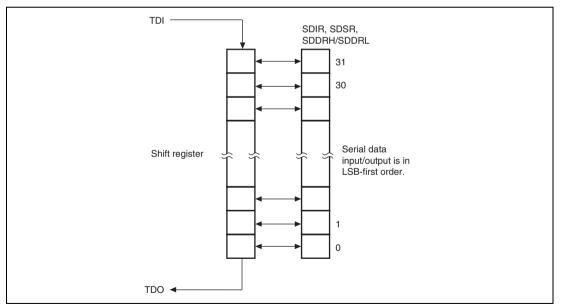
Figure 22.5 Serial Data Input/Output
