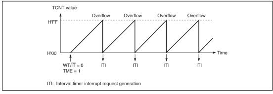
Figure 12.3 Operation in Interval Timer Mode
