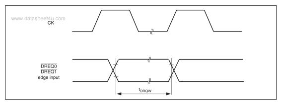
Figure 26.13 DREQ0, DREQ1 Input Timing (2)
