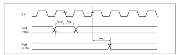
Figure 26.17 I/O Port Input/Output timing
