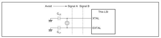
Figure 4.5 Cautions for Oscillator Circuit Board Design
