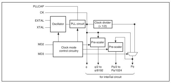
Figure 4.1 Block Diagram of Clock Pulse Generator
