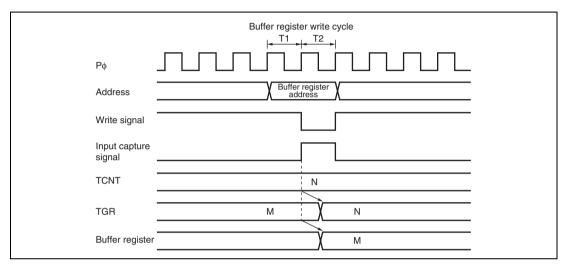
Figure 11.78 Contention between Buffer Register Write and Input Capture
