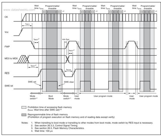
Figure 19.13 Mode Transit Timing (Example: Boot Mode → User Mode ⇔ User Program Mode)
