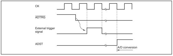
Figure 15.3 External Trigger Input Timing
