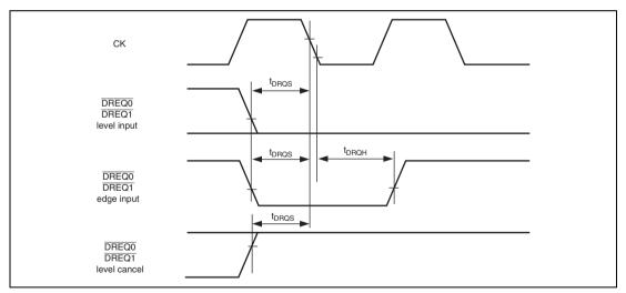
Figure 26.12 DREQ0, DREQ1 Input Timing (1)
