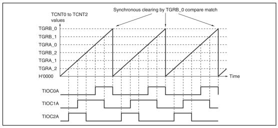
Figure 11.12 Example of Synchronous Operation
