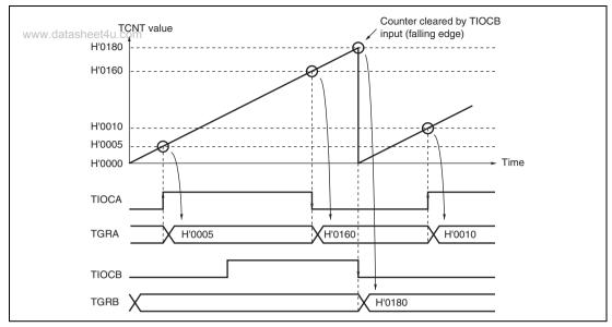
Figure 11.10 Example of Input Capture Operation
