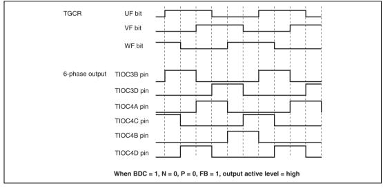
Figure 11.52 Example of Output Phase Switching by Means of UF, VF, WF Bit Settings
