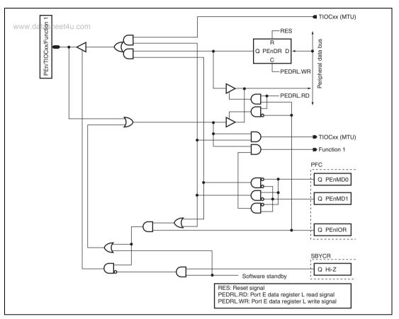
Figure D.34 PEn/TIOCxx/Function 1
