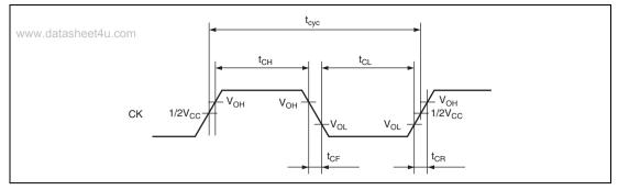
Figure 26.2 System Clock Timing
