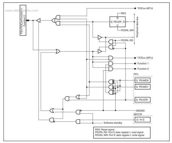
Figure D.43 PEn/TIOCxx/Function 1/Function 2
