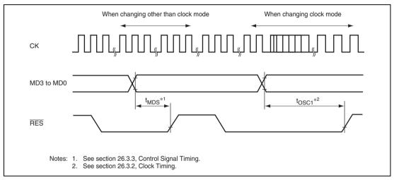
Figure 3.2 Reset Input Timing when Changing Operating Mode
