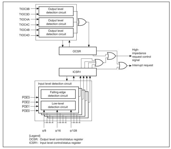
Figure 11.114 POE Block Diagram
