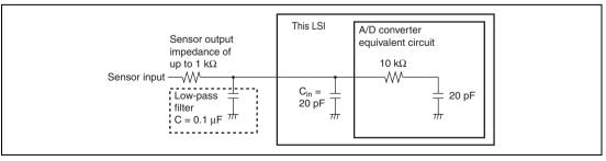
Figure 15.6 Example of Analog Input Circuit
