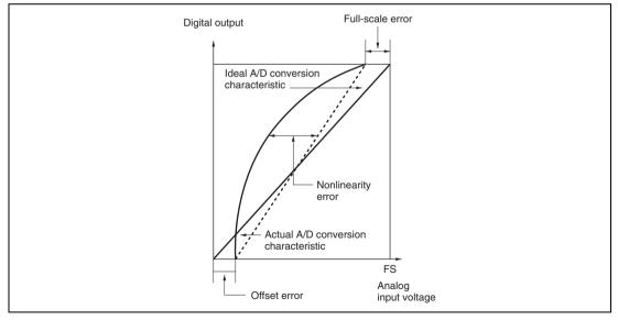
Figure 15.5 Definitions of A/D Conversion Accuracy
