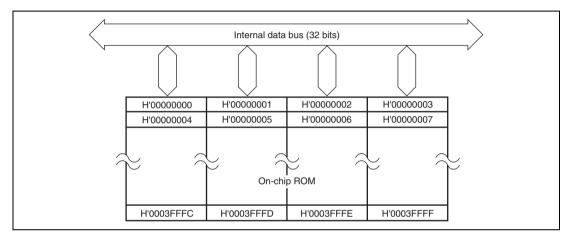
Figure 20.1 Mask ROM Block Diagram
