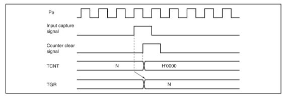
Figure 11.61 Counter Clear Timing (Input Capture)
