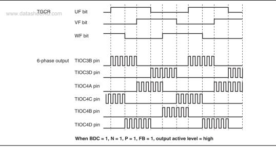
Figure 11.53 Example of Output Phase Switching by Means of UF, VF, WF Bit Settings (2)
