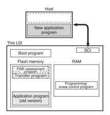
Writing new application program Next, the new application program in the host is written into the erased flash memory blocks. Do not write to unerased blocks.
