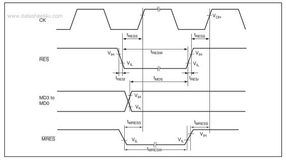
Figure 26.5 Reset Input Timing
