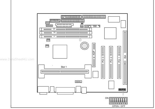
Switch 1 = must be set to *off* Switch 2 = System BIOS recovery (RCV) Switch 3 = Write protection for floppy disks Switch 4 = reserved Switches 5 - 8 = clock frequency
